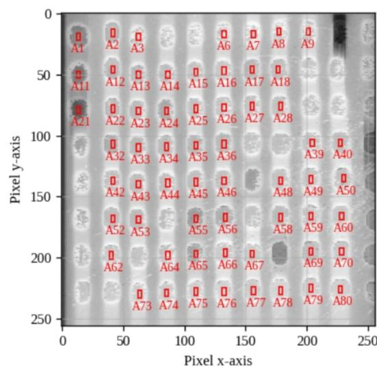
**Figure 11.** Arrangement of smell-sensitive membranes with good properties, which are circled in red and numbered Area 1 (A1) through Area 80 (A80).
