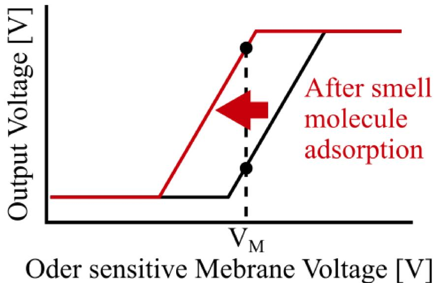
Figure 5. Shift in threshold voltage.
