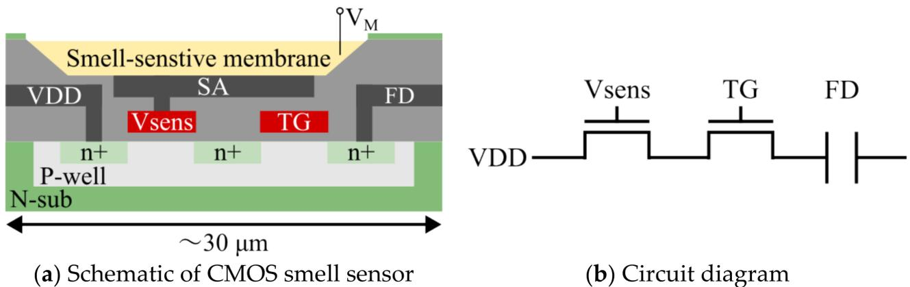
Figure 4. CMOS smell sensor.
