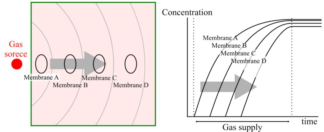
Figure 8. Proposal 1: a method for capturing diffusion velocity.
