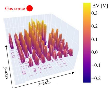
Figure 14. Three-dimensional map of voltage changes from 180 s to 240 s.
