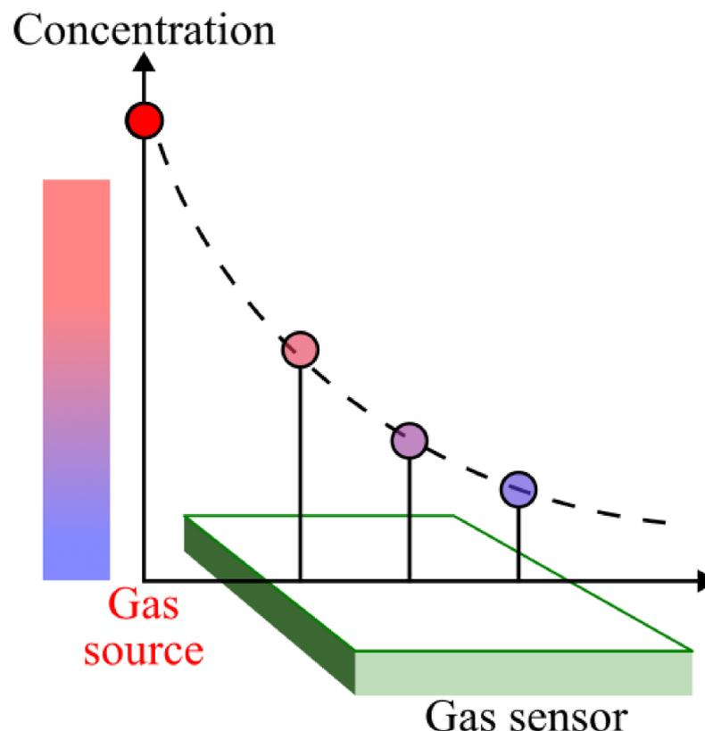
**Figure 1.** Principle of gas-source location estimation.
