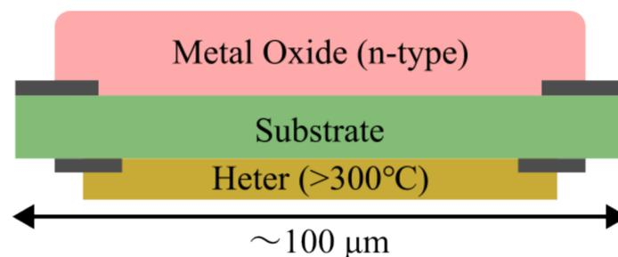
**Figure 3.** Schematic of semiconductor gas sensor.
