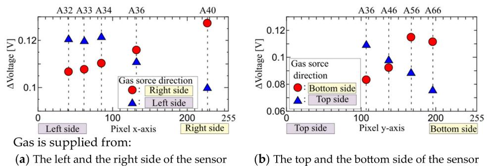
**Figure 16.** Voltage difference at the pixel position of the selected membranes.
