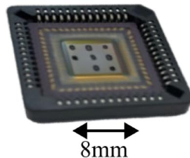
Figure 7. CMOS smell sensor array.
