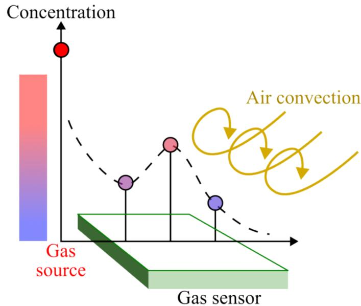
**Figure 2.** Estimation of gas-source location during air convection.
