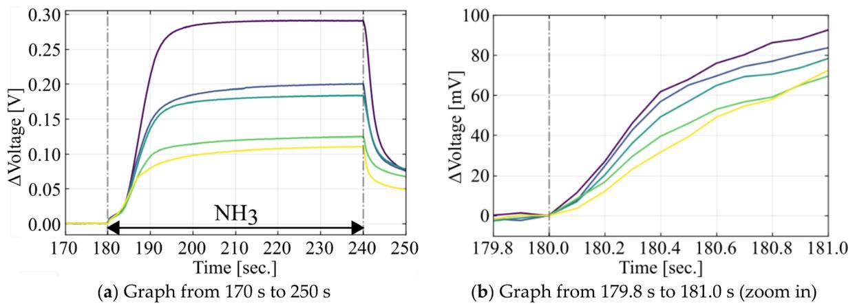
Figure 13. Output voltage characteristics of the membrane specified in Figure 12. Note that the solid line in the graph corresponds to the color of the membrane location in Figure 12.
