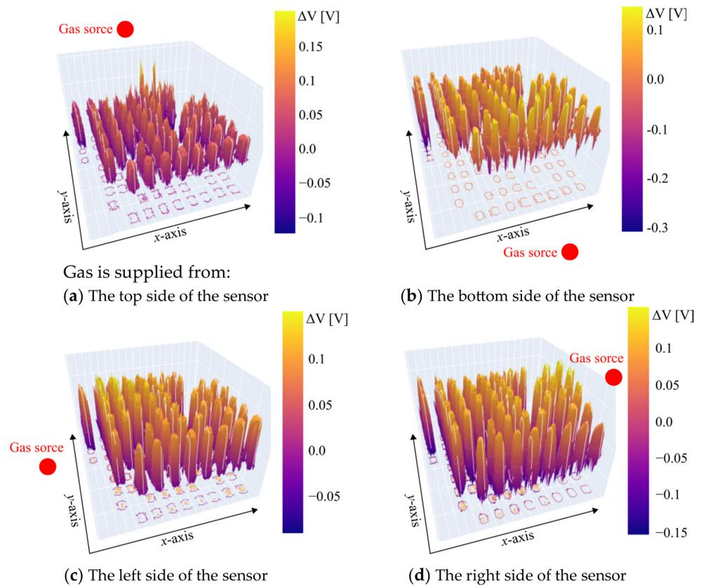
**Figure 15.** Three-dimensional map of voltage changes when gas is supplied from different sides.
