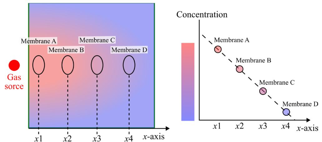
Figure 9. Proposal 2: method for capturing concentration gradients.
