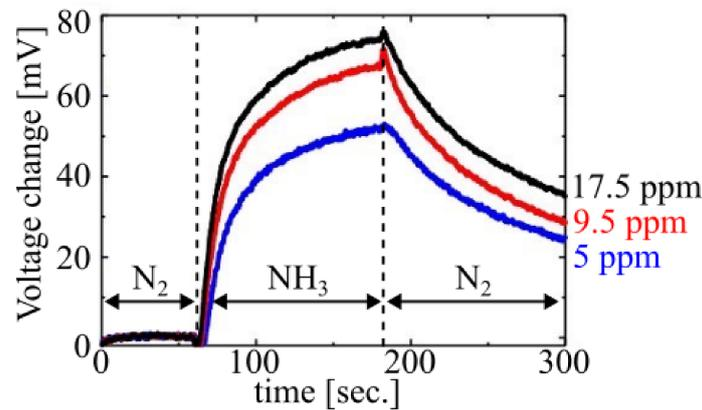
Figure 6. Example of CMOS smell sensor output voltage.
