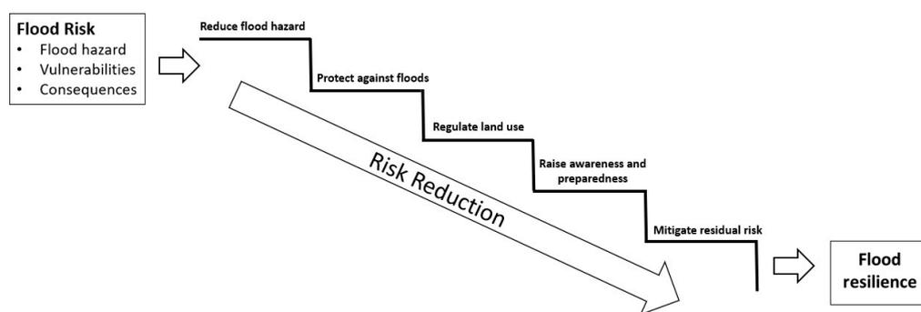
**Figure 1.** Cascade diagram of IFM measures.
