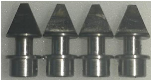
**Figure 23.** Photograph comparing erosion in tungsten–molybdenum-alloy jet vanes.
