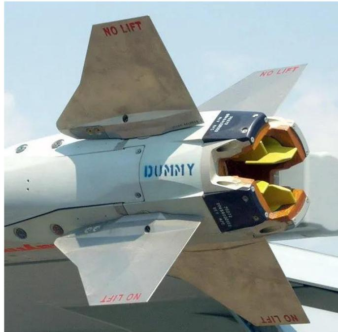
**Figure 4.** The jet-vane system of the AIM-9X missile.
