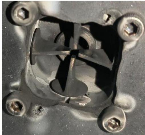
**Figure 22.** The condition of tungsten–molybdenum-alloy jet vanes after testing.
