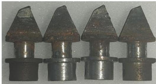
**Figure 16.** Photograph comparing erosion in 45 steel jet vanes.
