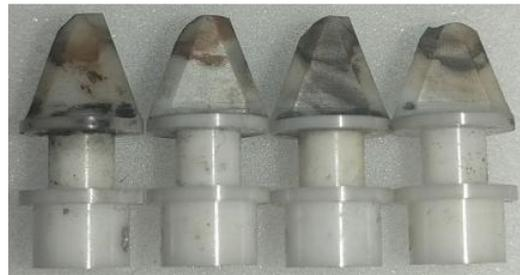
**Figure 20.** Photograph comparing erosion in alumina-ceramic jet vanes.
