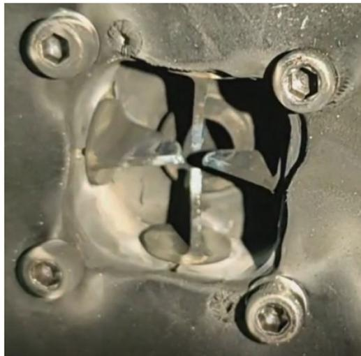
**Figure 15.** Condition of the 45 Steel jet vanes after testing.
