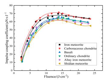
**Figure 6.** Comparison of impulse coupling curves of six types of asteroid simulants (the beam size was approximately 500  $\mu$ m at  $1/e^2$ , and the laser pulse duration was 10 ns).
