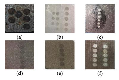
**Figure 3.** Ablation spots of six types of asteroid simulants: (**a**) carbonaceous chondrite; (**b**) iron meteorite; (**c**) basalt; (**d**) Shidian meteorite; (**e**) ordinary chondrite; (**f**) Altay iron meteorite.
