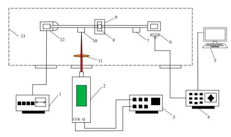
**Figure 2.** Schematic diagram of the experimental system. (1) Programmable power supply; (2) the Q-switched Nd:YAG laser; (3) digital pulse generator; (4) data acquisition unit; (5) computer; (6) displacement sensor; (7) counterweight block; (8) pivot; (9) two-dimensional displacement platform; (10) target material; (11) optical lens; (12) damper; (13) vacuum chamber.
