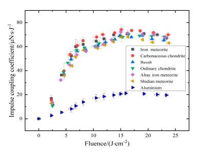
**Figure 5.** Impulse coupling coefficient of six types of asteroid simulants and the aluminum irradiated by different laser fluences (the beam size was approximately 500  $\mu$ m at  $1/e^2$ , and the laser pulse duration was 10 ns).
