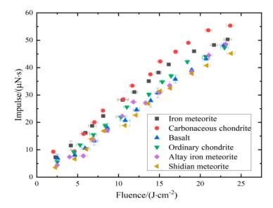
**Figure 4.** Impulse of six types of asteroid simulants irradiated by different laser fluences (the beam size was approximately 500  $\mu$ m at 1/e<sup>2</sup>, and the laser pulse duration was 10 ns).
