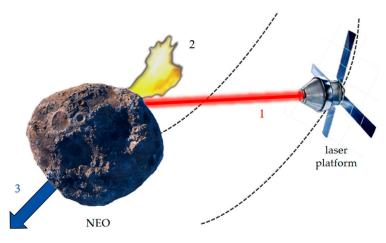
**Figure 1.** Schematic diagram of laser ablation deflection technology. (1) A high-power laser beam emitted by the laser platform; (2) ejecta plume of the surface material of the asteroid; (3) reaction force generated by the ejecta plume.
