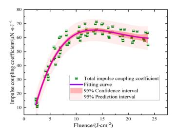
**Figure 7.** Fitting curves for the impulsive coupling characteristics of six types of asteroid simulants (the beam size was approximately 500  $\mu$ m at  $1/e^2$ , and the laser pulse duration was 10 ns).
