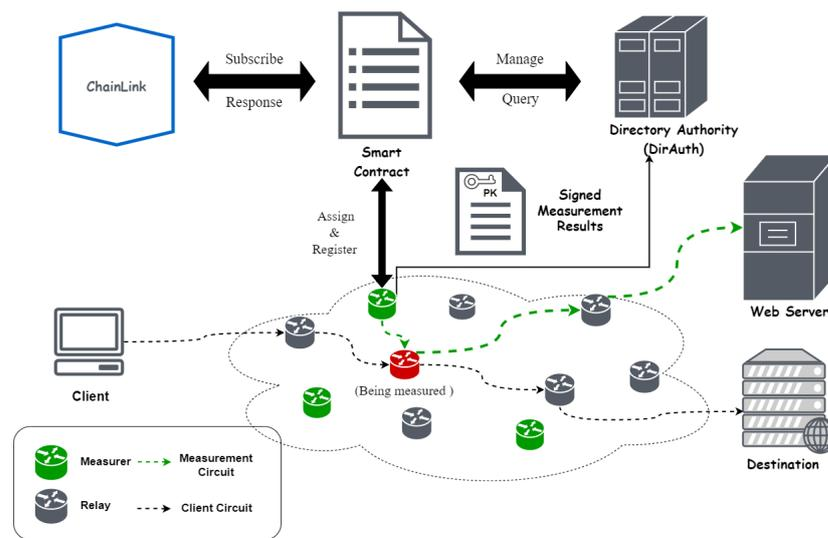
**Figure 1.** System Overview of SmartMeasurer. The red relay is being measured.
