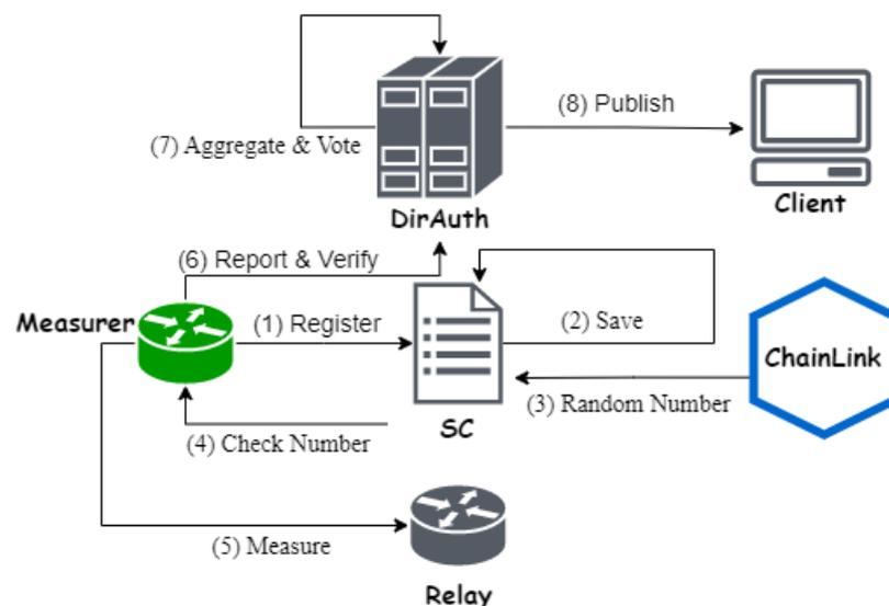
Figure 2. Work Process of SmartMeasurer.
