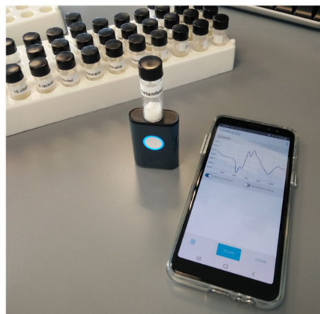
Figure 10. Handheld NIR spectrometer using a smartphone and scanning procedure for a SCiO NIR sensor with the glass sample vial placed directly on top of the light source and detection window. Reprinted with permission from reference [115].
