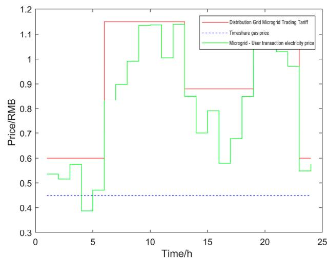
**Figure 7.** Electricity sales plan for microgrid users.
