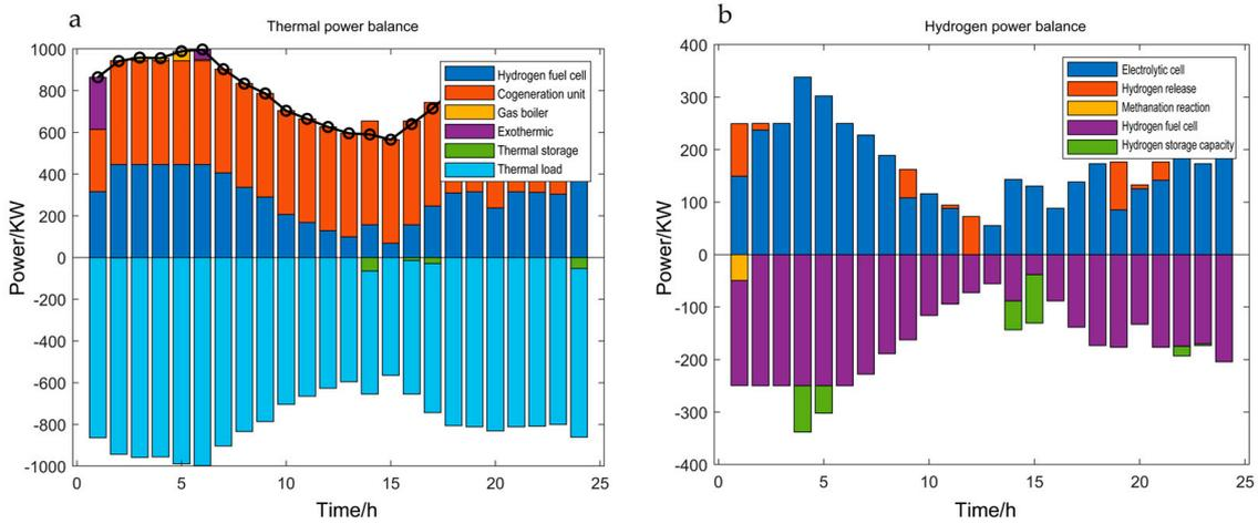
Figure 11. Device operation after demand response. (a) Thermal balance. (b) Hydrogen balance.
