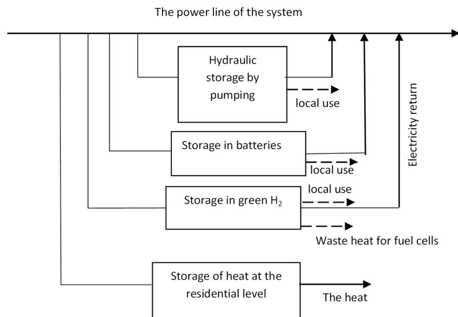
**Figure 1.** Schematic of the accumulation of electricity from the surplus period.
