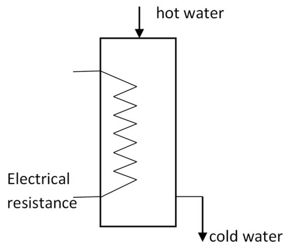
**Figure 3.** Schematic of the electric energy storage boiler in hot water.
