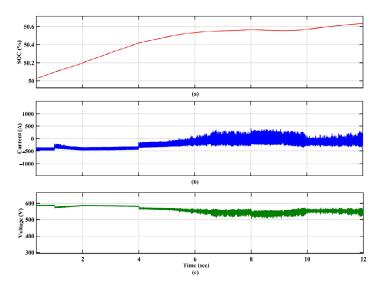
Figure 16. ESU (a) SOC, (b) current, and (c) voltage with the proposed controller.
