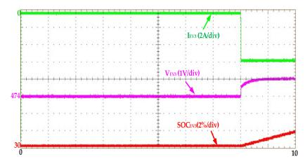
Figure 26. RT lab results for EV<sub>3</sub> SOC, voltage, and current with the proposed controller.
