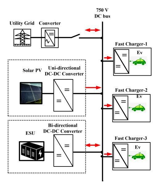
Figure 1. Schematic view of proposed microgrid-based DC fast charging station.
