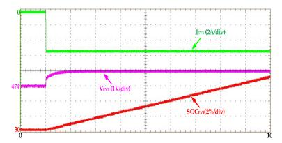
Figure 24. RT lab results for EV<sub>1</sub> SOC, voltage, and current with the proposed controller.
