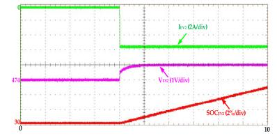
Figure 25. RT lab results for EV<sub>2</sub> SOC, voltage, and current with the proposed controller.
