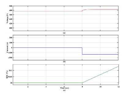
Figure 20. EV<sub>3</sub> (a) voltage, (b) current, and (c) SOC with the proposed controller.
