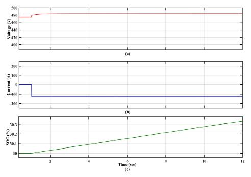
**Figure 11.** EV<sub>1</sub> (**a**) voltage, (**b**) current, and (**c**) SOC with MPPT controller.
