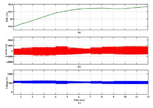
Figure 9. ESU (a) SOC, (b) current, and (c) voltage with MPPT controller.
