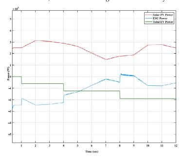
Figure 17. Power sharing with the proposed controller.
