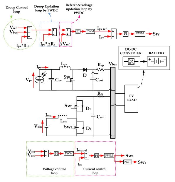
Figure 2. Control structure of solar PV and ESU.
