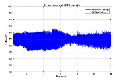
Figure 7. DC bus voltage with MPPT controller.
