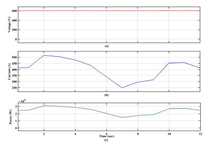
**Figure 15.** Solar PV (a) voltage, (b) current, and (c) power with the proposed controller.
