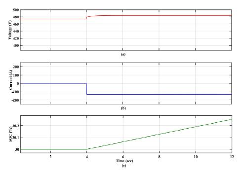
Figure 12.  $EV_2$  (a) voltage, (b) current, and (c) SOC with MPPT controller.
