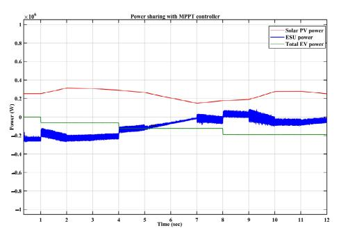
Figure 10. Power sharing with MPPT controller.
