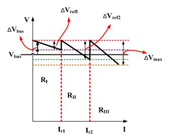
Figure 4. Piece-wise droop curve for three regions with voltage compensation.
