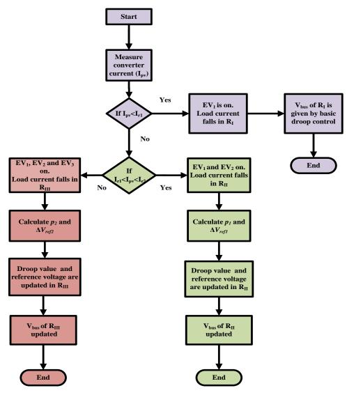
**Figure 5.** Flowchart of the proposed piece-wise droop control for three regions along with voltage compensation. Different colours represents different regions of the pice-wise droop curve.
