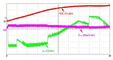
Figure 23. RT lab results for ESU SOC, voltage, and current of FEVCS with the proposed controller.
