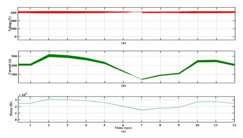
Figure 8. Solar PV (a) voltage, (b) current, and (c) power with MPPT controller.
