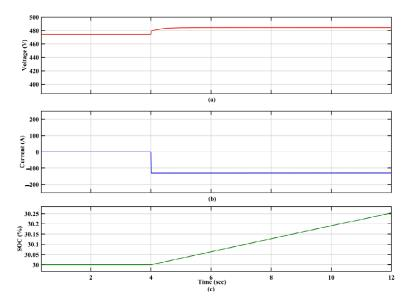
Figure 19. EV<sub>2</sub> (a) voltage, (b) current, and (c) SOC with the proposed controller.
