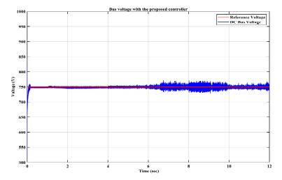
Figure 14. DC bus voltage with the proposed controller.
