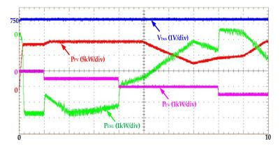
Figure 21. RT lab results for bus voltage and power sharing of FEVCS with the proposed controller.
