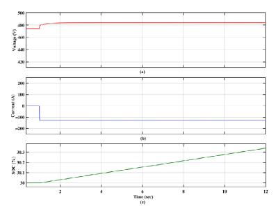
**Figure 18.**  $EV_1$  (a) voltage, (b) current, and (c) SOC with the proposed controller.
