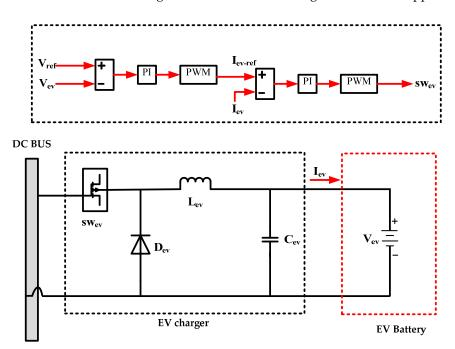
Figure 3. Control configuration of DC fast charger to charge the EV batteries.
