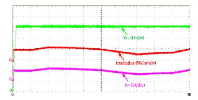
**Figure 22.** RT lab results for solar PV input irradiation, voltage, and current of FEVCS with the proposed controller.
