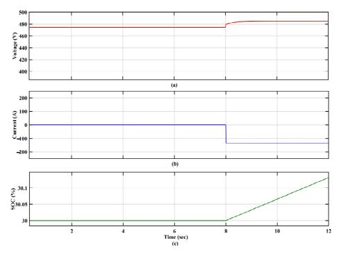
Figure 13.  $EV_3$  (a) voltage, (b) current, and (c) SOC with MPPT controller.
