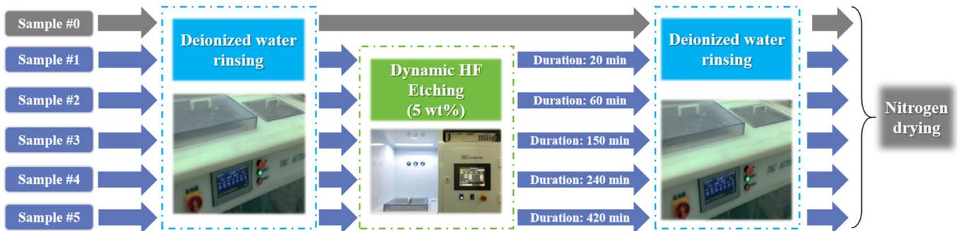
Figure 3. Etching schedule of each sample.
