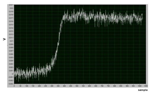
**Figure 3.** An event corresponding to the data-taking period of July–September 2021 is shown, in which the intrinsic noise of the digitizer at 4 mV is evident.
