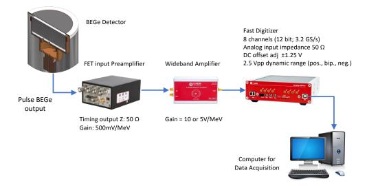
Figure 4. Block diagram of the upgraded BEGe DAQ system.
