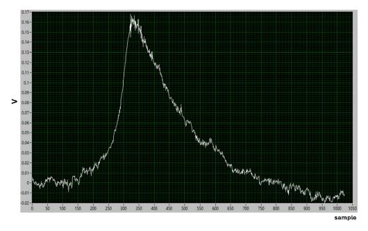
**Figure 5.** An event acquired during the 2022 data-taking period is shown: the peak-to-peak electronic noise corresponds to about 0.5 mV.
