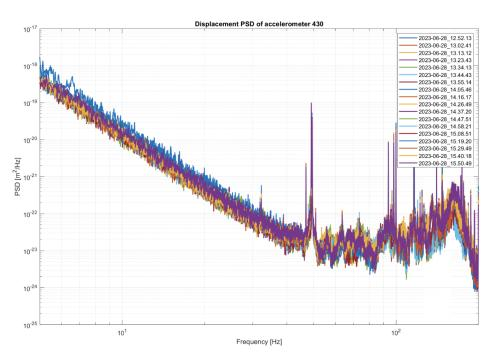
**Figure 7.** The results of a long-term measurement of the environmental noise in the laboratory is shown. The plot reports multiple measurements performed with one accelerometer and taken at consecutive times.
