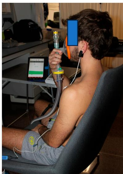
**Figure 2.** Participant holding the mask with his right hand, with a pulse oximeter on the left earlobe and Humon Hex® on the right thigh with the tablet to collect information on the evolution of SmO<sub>2</sub>.
