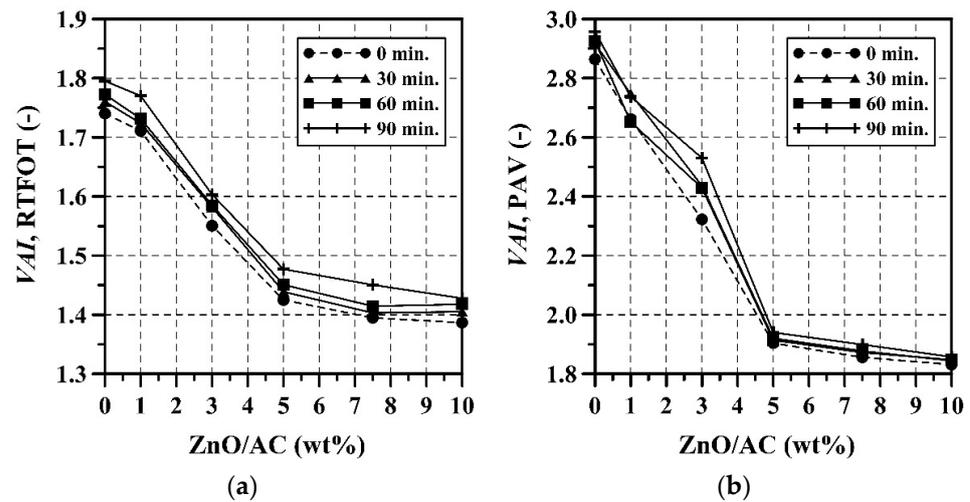
Figure 6. Evolution of VAI with ZnO/AC content and MT. (a) RTFOT, and (b) PAV.
