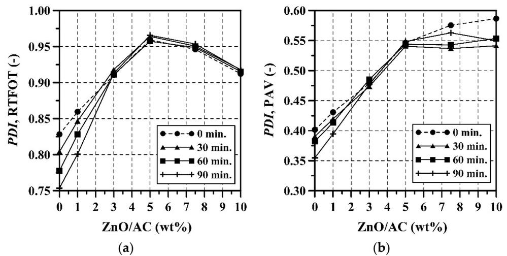
Figure 4. Evolution of PDI with ZnO/AC content and MT. (a) RTFOT, and (b) PAV.
