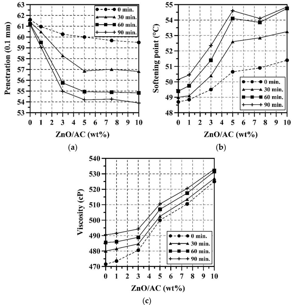
Figure 3. Evolution of (a) penetration, (b) softening point, and (c) viscosity with ZnO/AC content and MT.
