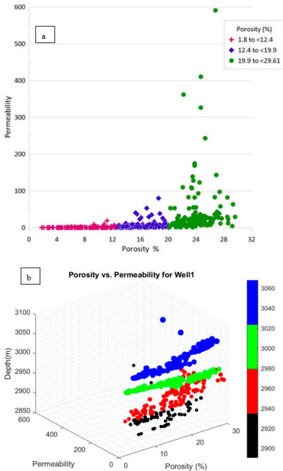
**Figure 3.** (a) Porosity–permeability relationship shown through a magnified image of the three porous–permeable zones; (b) 3D lattice form showing the porosity–permeability–depth relationship in Am1. Depth is provided in meters (m), porosity is given as a percentage (%), and permeability is presented in millidarcies (md).
