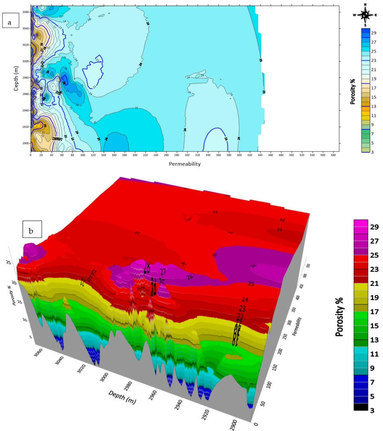
**Figure 6.** Subsurface distribution map for porosity and permeability range zones in (a) 2D and (b) 3D. Depth is provided in meters (m), porosity is given as a percentage (%), and permeability is presented in millidarcies (md).
