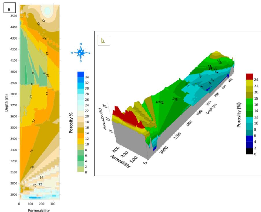
**Figure 5.** Subsurface distribution map for porosity and permeability range zones in (a) 2D and (b) 3D. Depth is provided in meters (m), porosity is given as a percentage (%), and permeability is presented in millidarcies (md).
