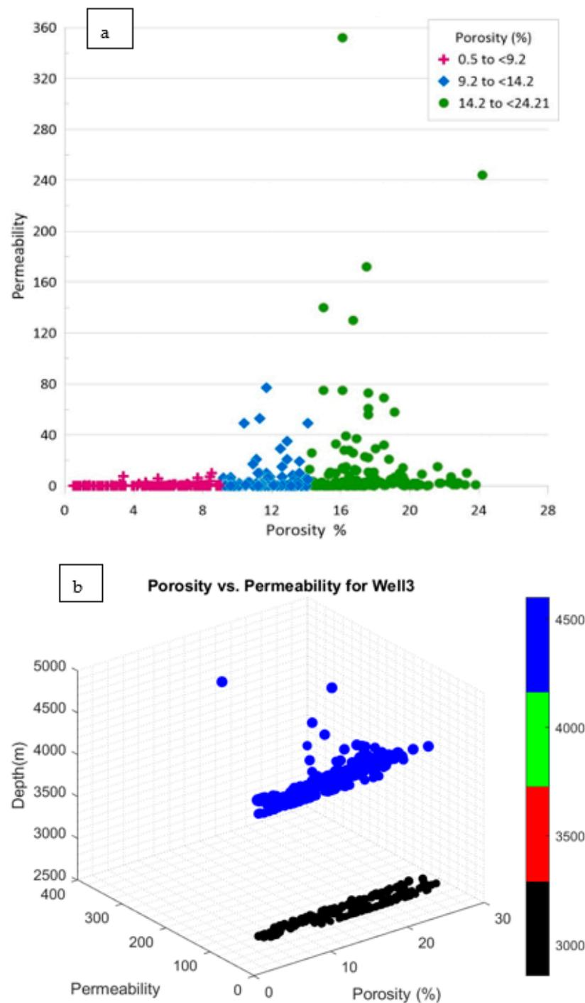
**Figure 4.** (a) Porosity–permeability relationship shown through a magnified image of the three porous–permeable zones; (b) 3D lattice showing the porosity–permeability–depth relationship in Am3. Depth is provided in meters (m), porosity is given as a percentage (%), and permeability is presented in millidarcies (md).
