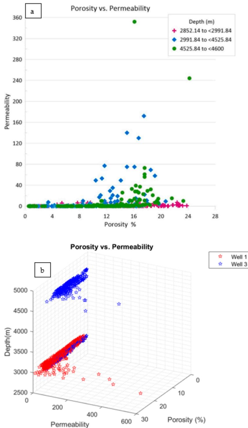
**Figure 7.** Subsurface distribution map for (a) porosity–permeability relationship and (b) porosity–permeability–depth in 3D form for Am1 and Am2. Depth is provided in meters (m), porosity is given as a percentage (%), and permeability is presented in millidarcies (md).
