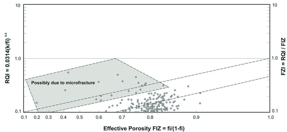
**Figure 2.** Log–log plot of the Reservoir Quality Index (RQI) versus effective porosity of the Khasib Formation. Data were obtained from wells in the East Baghdad field [9].
