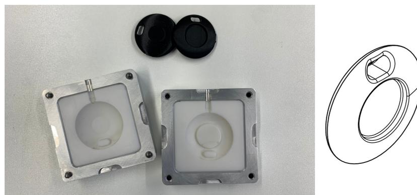
**Figure 8.** Fabricated 3D-printed mold for production of the chip key.
