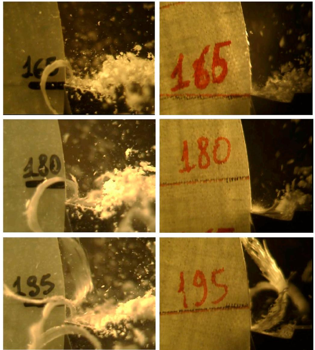
**Figure 18.** Chip morphology of circular specimens with (left) and without polycarbonate (right), around  $\theta = 180^\circ$  ( $\gamma = 15^\circ$ ,  $\alpha = 15^\circ$ ,  $a_c = 0.20$  mm, and  $v_c = 50$  m/min).
