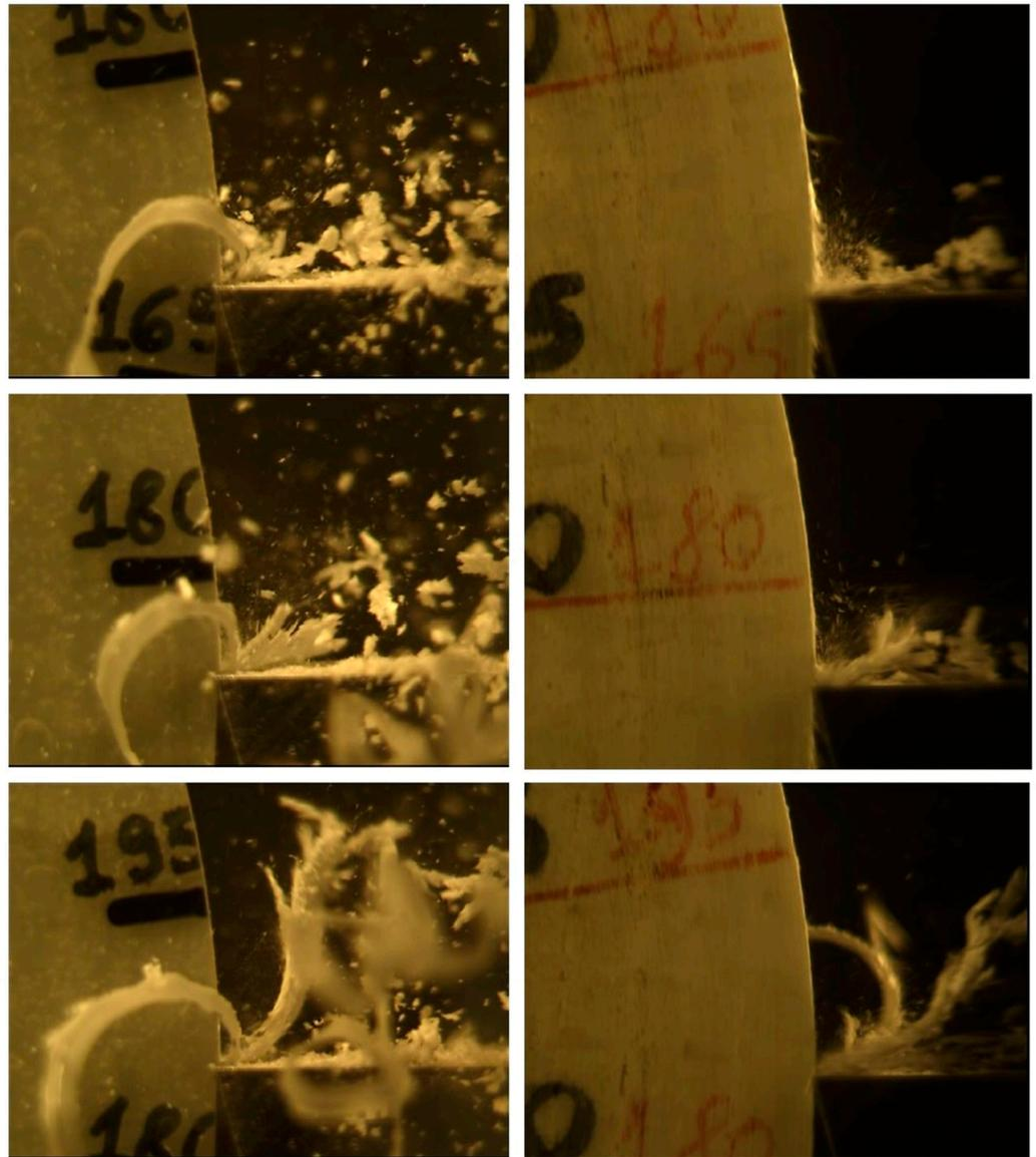
**Figure 17.** Chip morphology of circular specimens with (left) and without polycarbonate (right), around  $\theta = 180^\circ$  ( $\gamma = 0^\circ$ ,  $\alpha = 15^\circ$ ,  $a_c = 0.20$  mm, and  $v_c = 50$  m/min).
