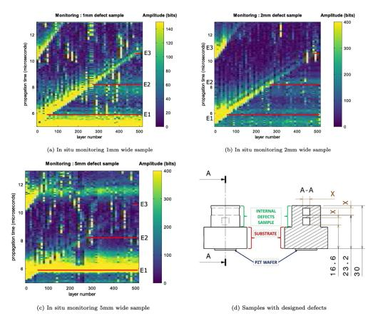
Figure 14. In situ monitoring of samples with internal designed defects [38].
