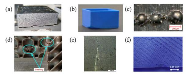
**Figure 1.** Typical examples of defects in additive manufacturing showing: macro-cracks (**a**) [23], warping (**b**) balling (**c**) [24], swelling (**d**) [25], micro-cracks (**e**) [26], and an under-filled part (**f**) [27].
