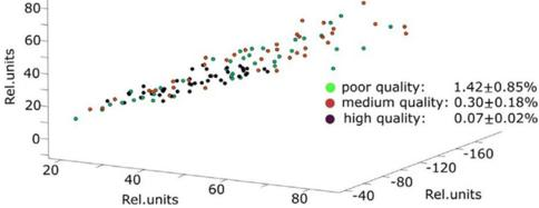
**Figure 16.** Projection of the acoustic features into a 3D feature space using principal component analysis (PCA) [40].
