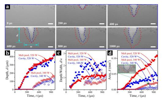
**Figure 3.** Dynamic changes in the melt pool during the laser powder bed fusion process of Ti-6Al-4V [29].
