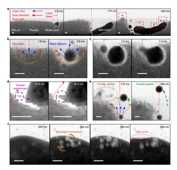
**Figure 8.** Time-series radiographs acquired during LAM of an Invar 36 single-layer melt track (MT1) under P = 209 W, v = 13 mm/s, and LED = 16.1 J/mm [32].
