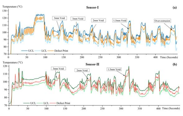
**Figure 10.** +/3σ control chart comparing defected print temperature data with control limits [34]. (a) Sensor-I and (b) Sensor-II.
