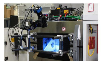
**Figure 4.** The camera setup in front of the LBM machine [30]. The modular tube construction enables flexible positioning with an adjustable height, position, and distance from the door.
