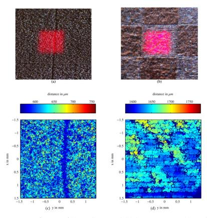
**Figure 7.** Surface scan of (**a**) powder material, (**b**) the SLM structure, (**c**) powder material, and (**d**) the SLM structure [31].
