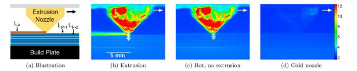
**Figure 9.** Illustration and false color IR images of 3D printing process. From left to right, (**a**) an illustration, (**b**) extrusion, a (**c**) hot extruder/no extruder, and (**d**) a cold extruder are shown (the color scale is linear) [33].
