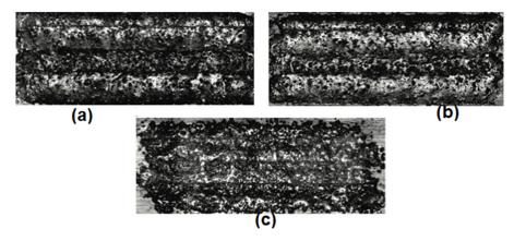
**Figure 13.** Stitched micrograph sample images of each build condition showing differing surface characteristics and surface breaking cracks. (**a**) Baseline condition, (**b**) surface roughness influenced by a low-laser-power setting, and (**c**) significant cracks and rips generated in a low-powder-flow scenario [37].
