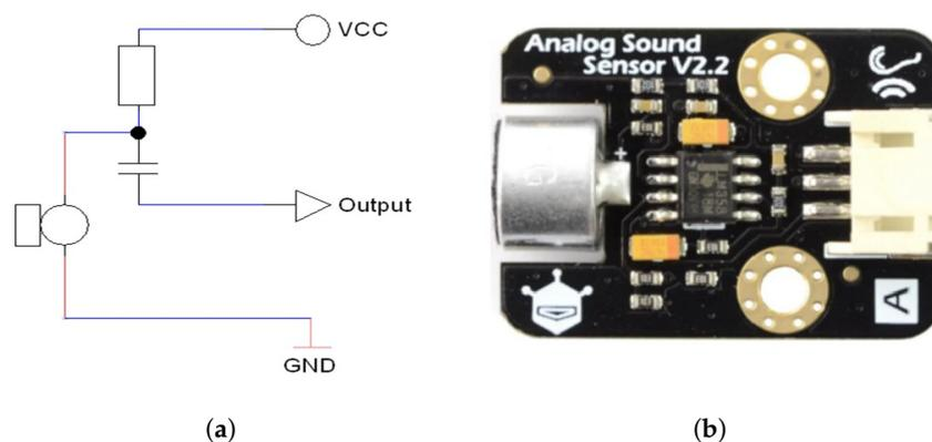
**Figure 6.** (a) Schematic diagram of an electret microphone pre-amplifier; (b) DFRobot Modul Analog Sound Sensor V2.2.
