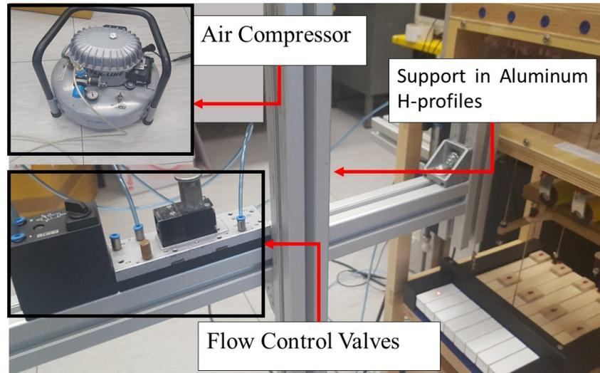
**Figure 5.** Pneumatic system: air compressor, pressure regulators, and valves on support.
