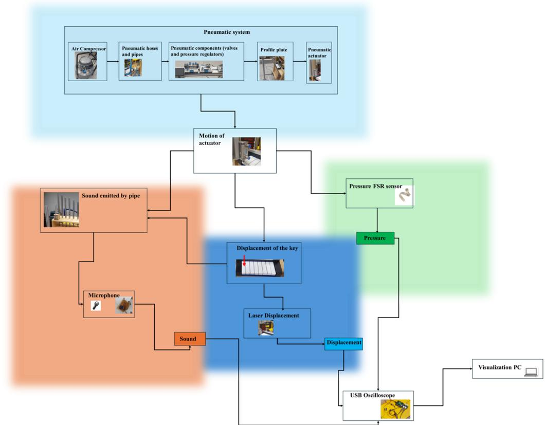
**Figure 3.** Diagram of the conducted measurements in the organ pipe.
