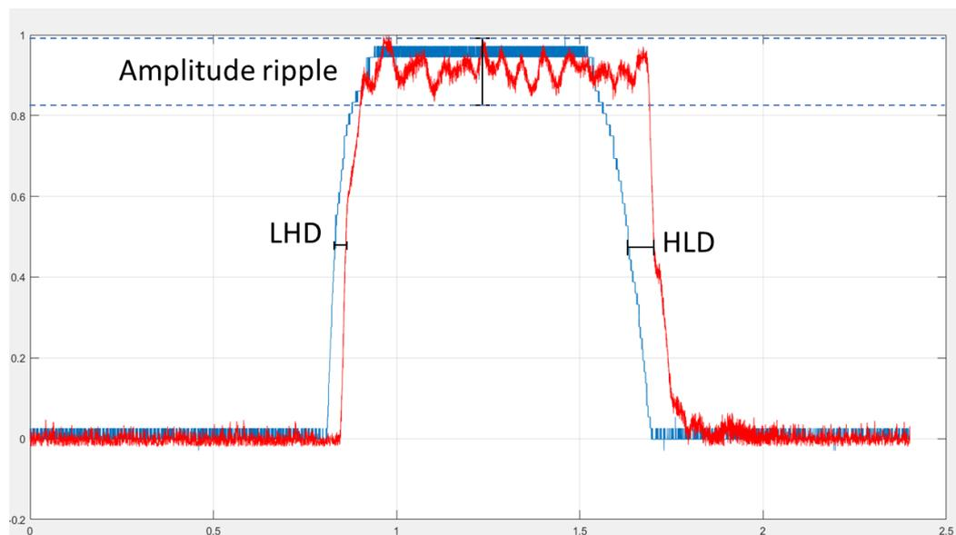
**Figure 14.** Amplitude ripple (AR), the low-to-high delay (LHD), and the high-to-low delay (HLD) of  $P^*(t)$  and  $P(t)$ .
