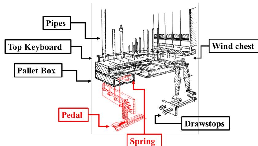
**Figure 1.** Mechanical organ instrument commonly used showing the mechanical traction with register cooperating with the tone and wind chest, pallet box, pedal, valve spring and the keyboard [34].
