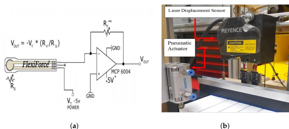
**Figure 7.** (a) Schematic diagram of the pressure sensor connected to the amplification circuit; (b) Laser Displacement Sensor and pneumatic actuator in organ pipe.
