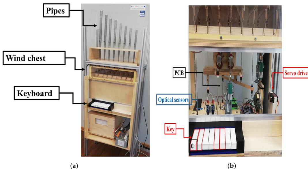
**Figure 2.** (a) A prototype of an organ instrument; (b) keyboard of organ instrument realized.
