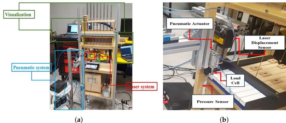
**Figure 8.** (a) Experimental setup of organ instrument and measurement apparatus; (b) laser displacement system, pneumatic actuator, flexible pressure sensor on musical keyboard.
