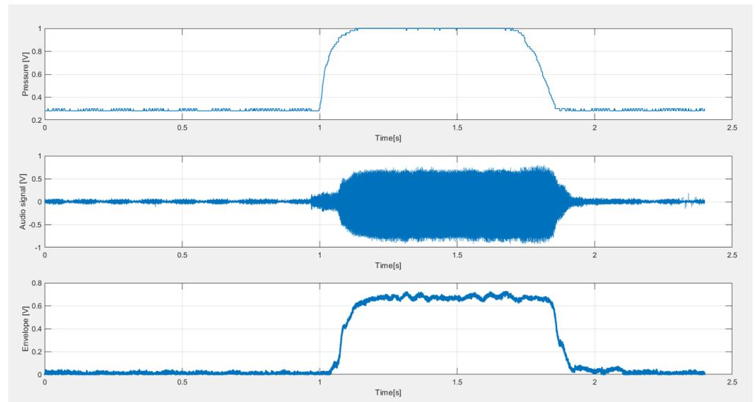
**Figure 13.** The first graph shows the pressure  $P(t)$ , the second, the audio signal generated by the pipe organ, and finally the last one,  $P^*(t)$  estimated by the computation of the absolute value of the Hilbert transform.
