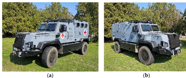
**Figure 4.** Autonomous vehicle type RDO 3927 KOMONDOR with a rescue (a) and reconnaissance (b) superstructure. Source: author's picture.
