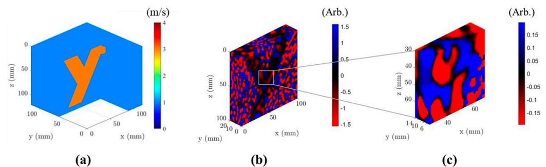
**Figure 2.** k-Wave elastography simulation: (a) SWS properties in the k-Wave simulation including a branching y-shaped tube in a uniform background (b) particle velocity field within the background material and y-shaped tube along the z-axis at a frequency of 200 Hz, (c) a focused view of particle velocity field within the y-shaped tube.
