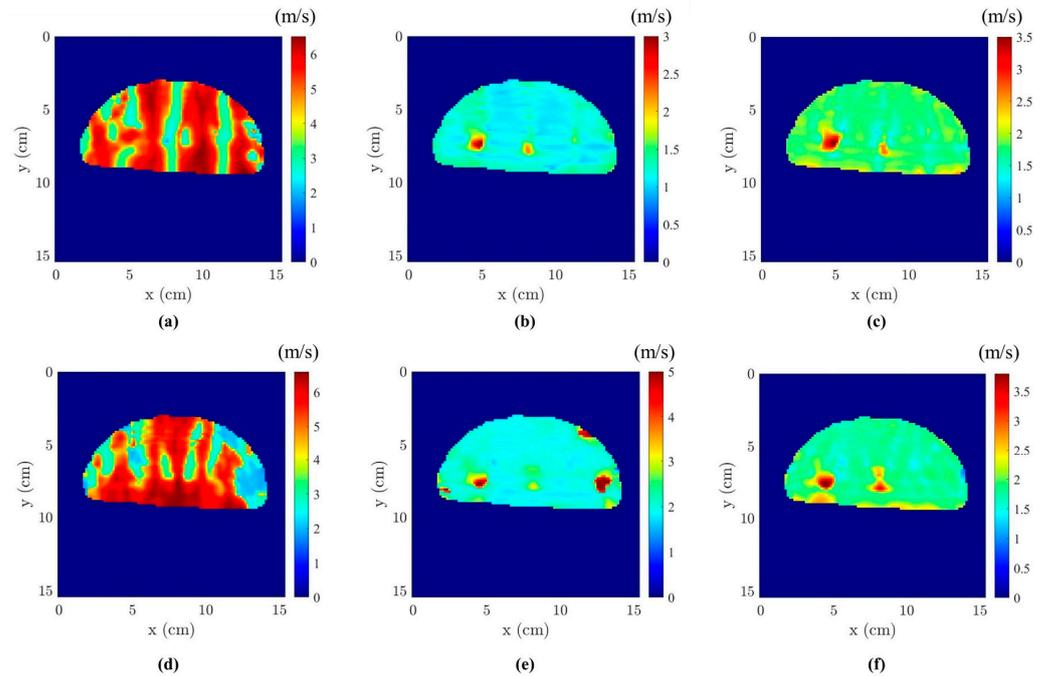
**Figure 11.** Estimated SWS of the brain-mimicking phantom with two lesions at the frequency of 200 Hz using (a) simple autocorrelation in  $x$ -direction, (b) simple autocorrelation in  $y$ -direction, and (c) the AIA approach on the X-motion MRE dataset. Estimated SWS using (d) simple autocorrelation in  $x$ -direction (e) simple autocorrelation in  $y$ -direction, and (f) the AIA approach on the Z-motion MRE dataset.
