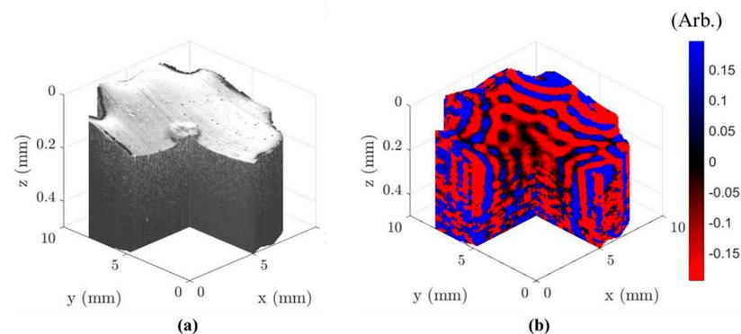
**Figure 6.** OCE of a phantom containing a lesion: (a) 3D OCT scan of the phantom with a pie-cut, (b) displacement field of shear waves at the frequency of 1500 Hz.
