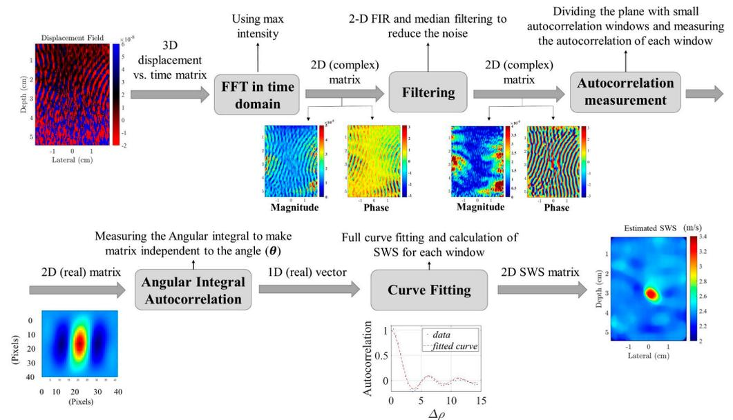
**Figure 1.** The algorithm for SWS estimation in ultrasound elastography of a phantom with a lesion.
