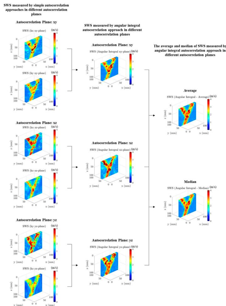
**Figure 7.** SWS measured from the k-Wave simulation at the frequency of 200 Hz using the simple baseline autocorrelation approaches in different planes and directions (left column), using the AIA approach in different autocorrelation planes (middle column), the average and median SWS measured by AIA approach in different autocorrelation planes (right column).
