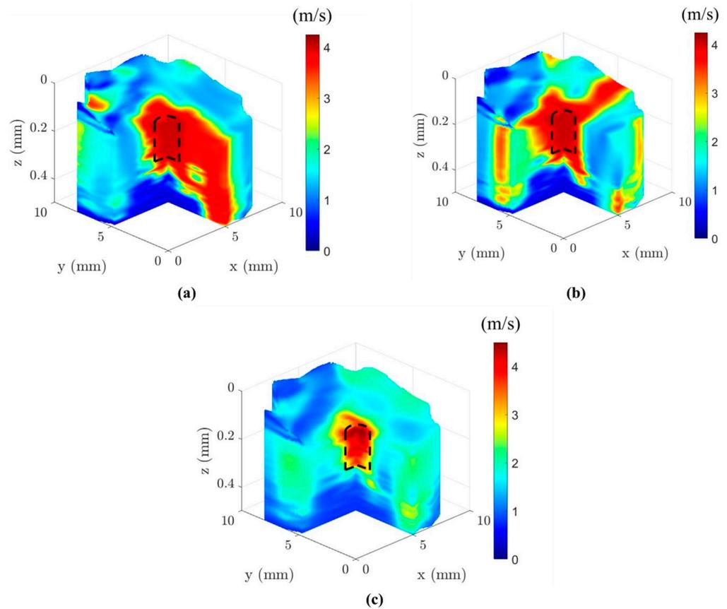
**Figure 12.** Comparative evaluation of estimated SWS for the OCE scan of the gelatin phantom with a lesion at the frequency of 1500 Hz using (a) simple autocorrelation approach in  $x$ -direction, (b) simple autocorrelation approach in  $y$ -direction, and (c) the AIA approach.
