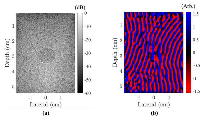
**Figure 3.** Ultrasound elastography of a breast phantom with a lesion at the center: (a) B-mode ultrasound scan of the phantom, (b) phase map of the shear-wave field at the frequency of 900 Hz.
