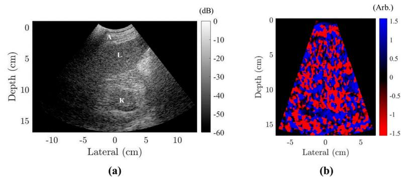
**Figure 4.** Ultrasound elastography of a human liver–kidney: (a) B-mode ultrasound scan of the human liver–kidney region including the abdominal layer (zone A), the liver (zone L), and the kidney (zone K), (b) phase map of the reverberant shear-wave field at the frequency of 702 Hz.
