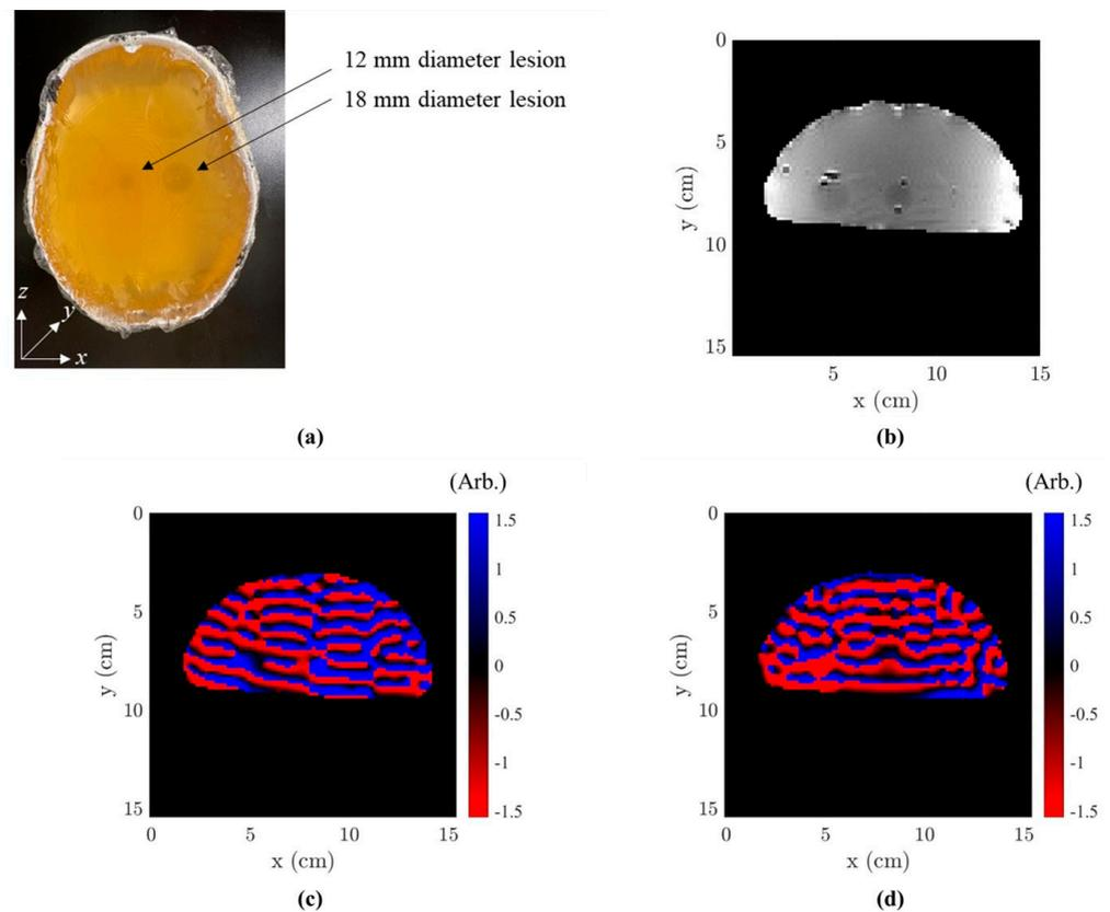
**Figure 5.** MRE of a brain phantom with two lesions: (a) brain phantom shape and the coordinate system for MRE, (b) MRI scan of the brain phantom (c) phase map of X-motion, and (d) phase map of Z-motion displacement fields at the frequency of 200 Hz.
