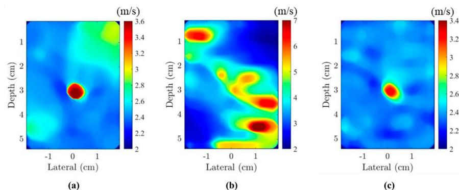
**Figure 8.** Estimated SWS using (a) simple autocorrelation in x-direction (b) simple autocorrelation in z-direction, and (c) the AIA approach for ultrasound elastography of a breast phantom with a lesion at the frequency of 900 Hz.
