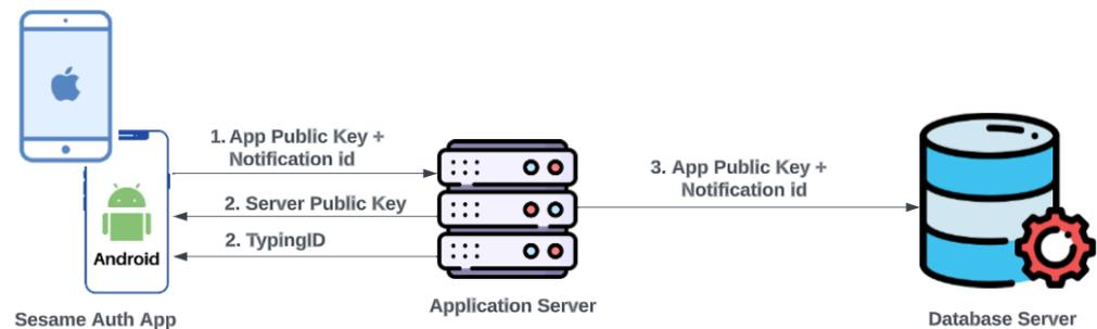
**Figure 2.** SA app installation process flow.
