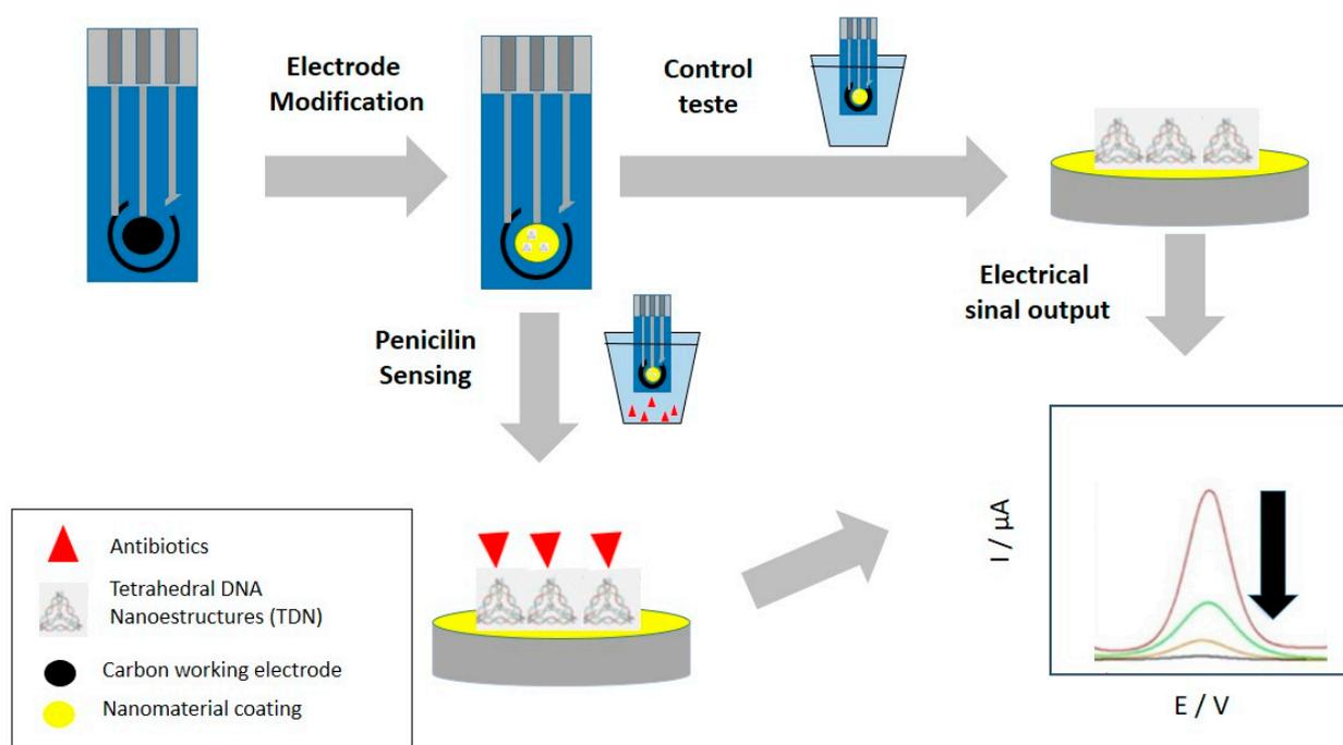
**Figure 4.** Illustration of penicillin detection with the electrochemical aptasensor (adapted from ref. [48]).
