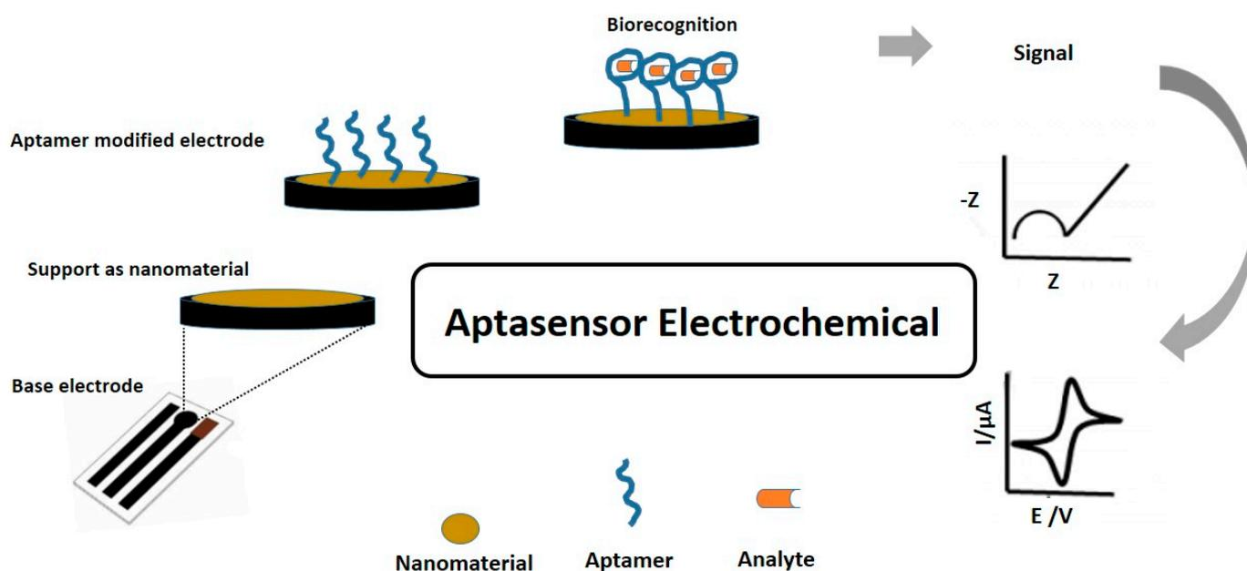
**Figure 3.** Electrochemical aptasensor illustration.
