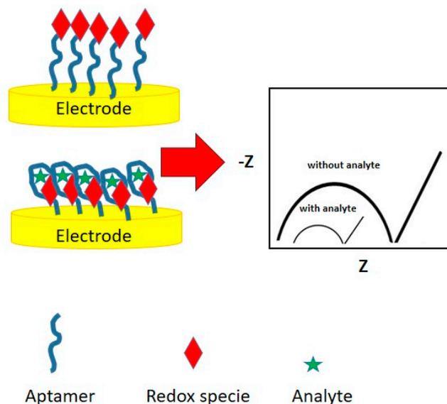
**Figure 5.** Illustration of label-based electrochemical aptasensor.
