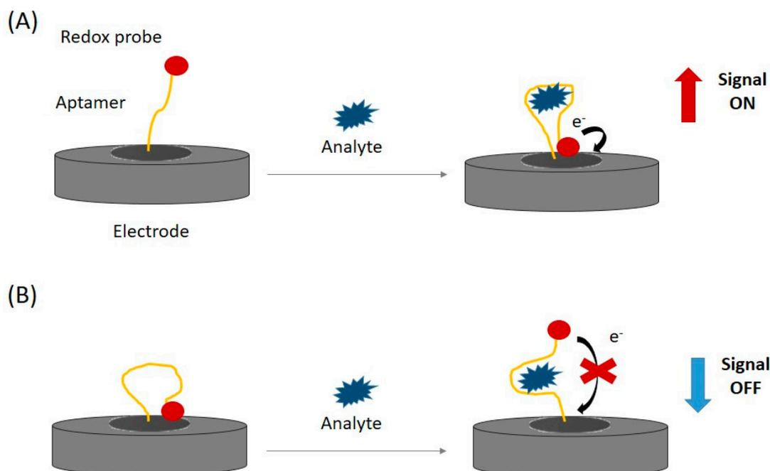
**Figure 6.** Design strategy based on “signal on/off” that occurs when aptamer interacts with an analyte. (A) Electrochemical aptasensor with off to on and (B) on to off (adapted from ref. [7]).
