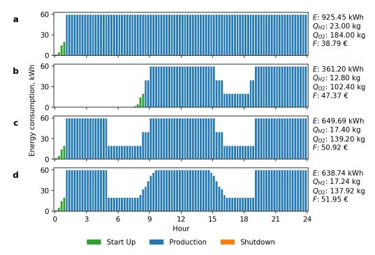
**Figure 2.** Electrolyser schedules compared (15 min resolution): (**a**) "full power" production, (**b**) the best schedule by MCTS, (**c**) the best schedule by CP-SAT model (fixed production levels) and (**d**) the best schedule by CP-SAT model (variable production levels).
