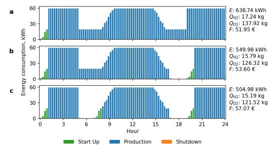
**Figure 3.** Electrolyser schedules depending on various amortisation costs per on–off cycle: (**a**) EUR 6.00 (baseline), (**b**) EUR 3.00 and (**c**) EUR 1.50.
