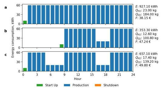
**Figure 1.** Electrolyser schedules compared (1 h resolution): (**a**) "full power" production, (**b**) the best schedule by MCTS and (**c**) the best schedule by CP-SAT model.
