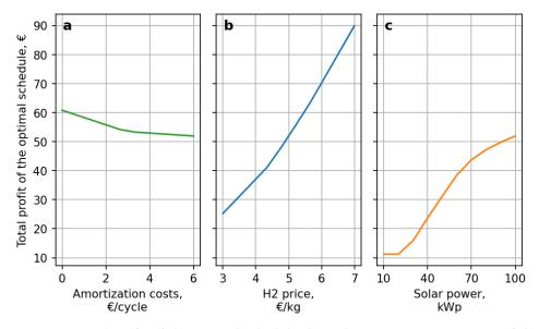
**Figure 5.** Total profit of the optimal schedule depending on input parameters of the model: (a) amortisation costs, (b)  $H_2$  price and (c) available solar power.
