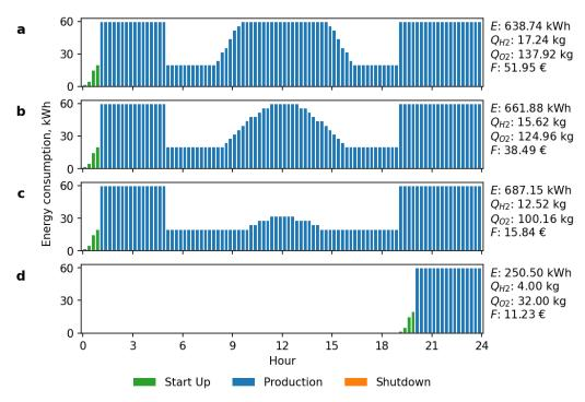
**Figure 4.** Electrolyser schedules depending on available renewable power (solar at peak): (**a**) 100 kWp (baseline), (**b**) 60 kWp, (**c**) 30 kWp and (**d**) 10 kWp.
