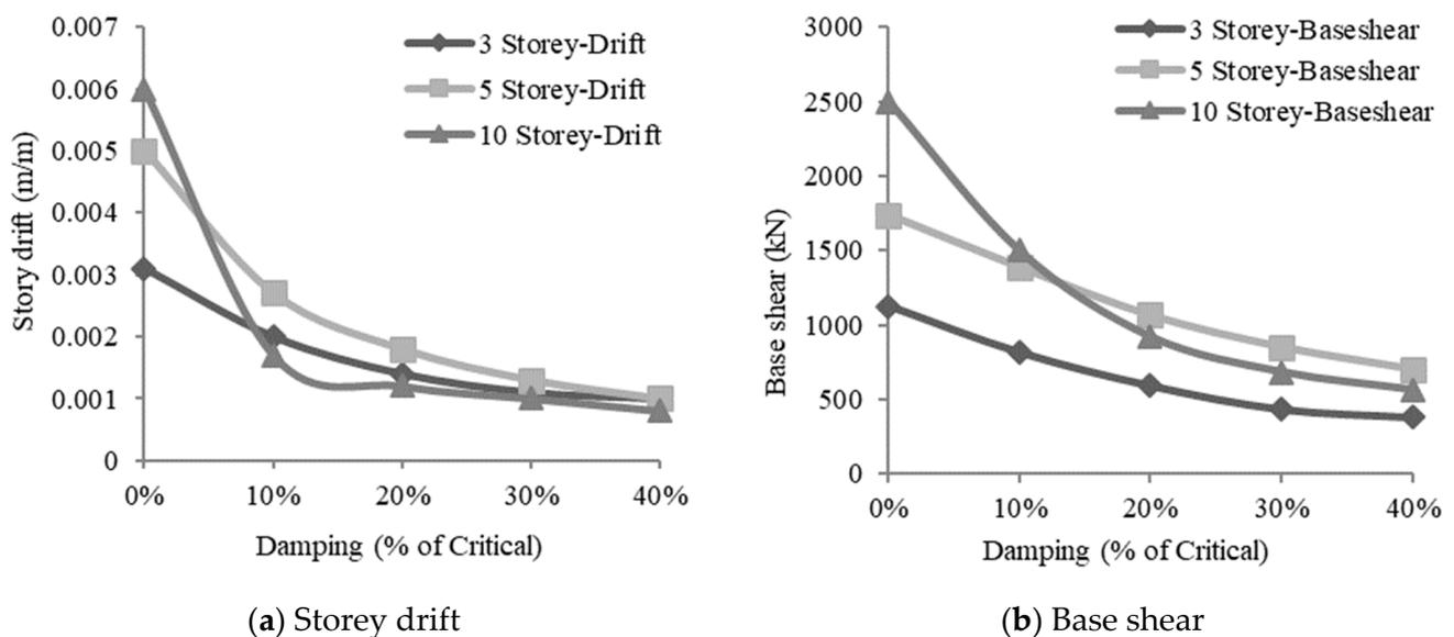
**Figure 4.** Effect of increases in the damping ratio: (a) storey drift, (b) base shear.
