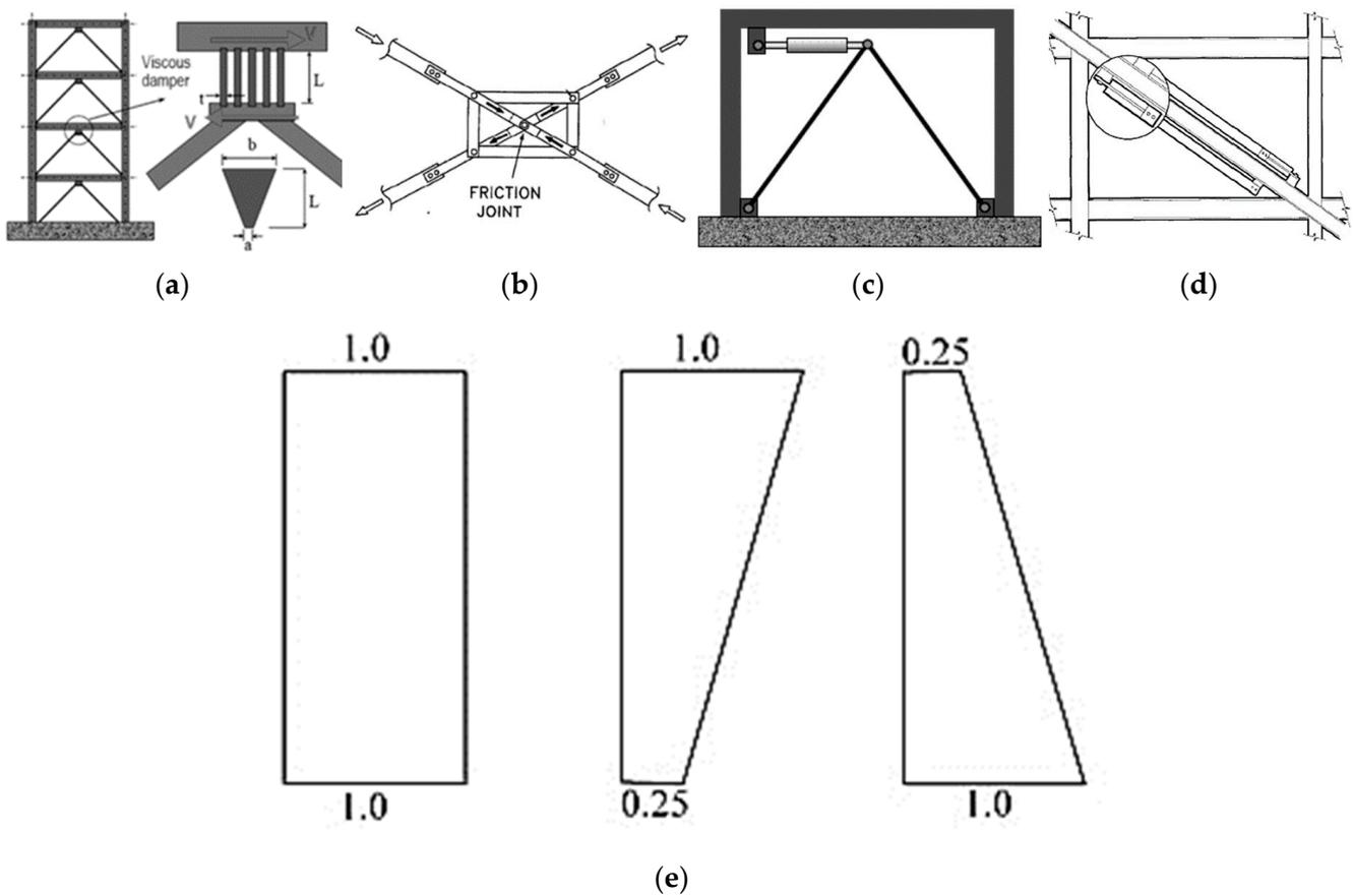
**Figure 2.** Dampers: (a) hysteretic, (b) friction, (c) viscous, and (d) viscoelastic; (e) parameter variations: uniform, reverse triangular, and triangular.
