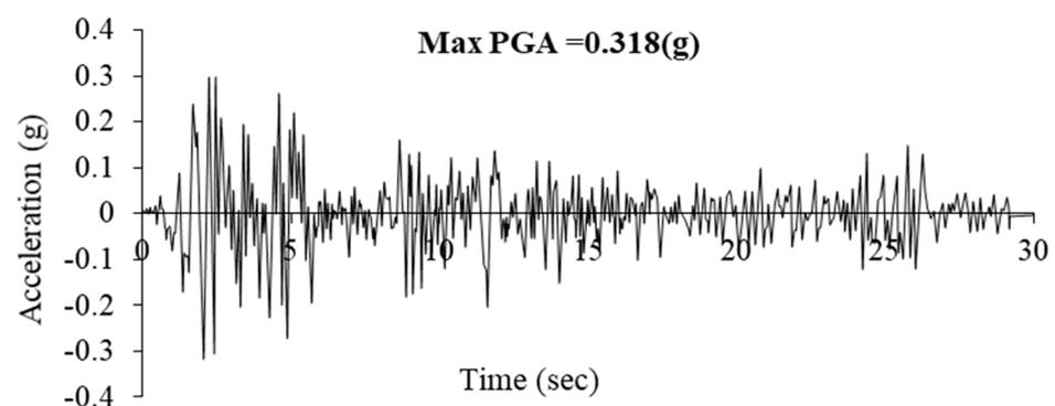
**Figure 1.** Time Acceleration Graph of the El Centro Earthquake in the E–W Direction.
