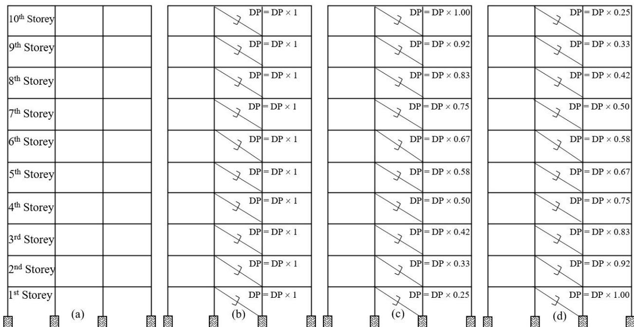
Figure 3. Damper parameter variation distribution with building height, (a) without dampers, (b) uniform, (c) triangular, and (d) reverse triangular.
