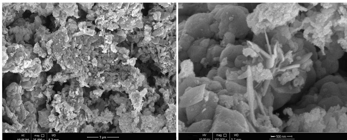
**Figure 4.** SEM images of the synthesized  $\text{Cu}_4\text{SnS}_4/\text{CuCo}_2\text{S}_4$ .
