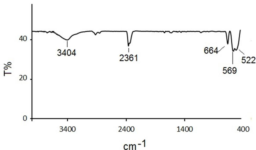
**Figure 1.** FT-IR spectrum of the synthesized Cu<sub>4</sub>SnS<sub>4</sub>/CuCo<sub>2</sub>S<sub>4</sub>.
