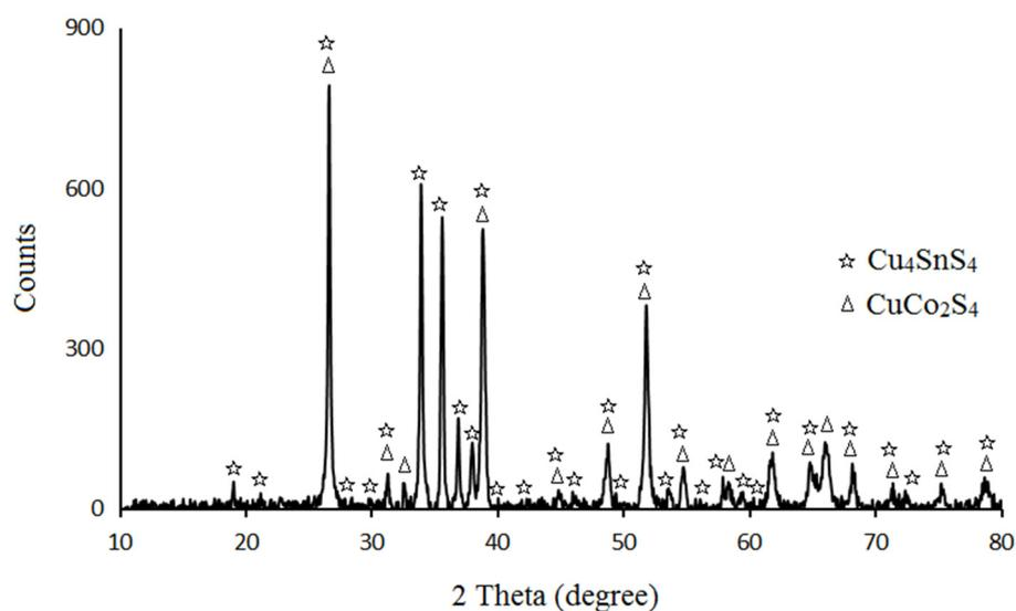
**Figure 2.** XRD pattern of the prepared Cu<sub>4</sub>SnS<sub>4</sub>/CuCo<sub>2</sub>S<sub>4</sub> nanoparticles.
