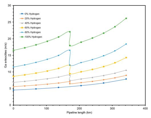
Figure 13. Gas velocities for compression option.
