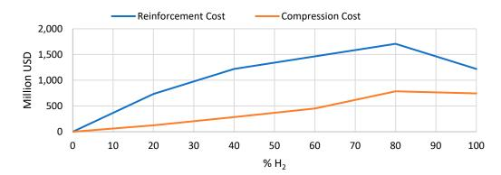
Figure 15. Comparison of pipeline expansion costs by looping versus compression.
