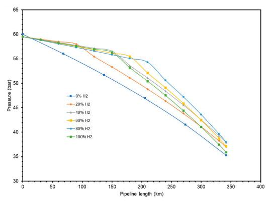
Figure 9. Pressure profile of the reinforced pipeline.
