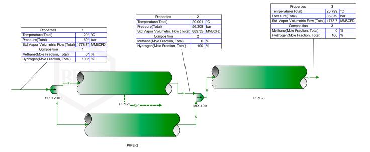
**Figure 7.** Process diagram of pipeline expansion with looping/pipe reinforcement (\* denoting a feed stream).
