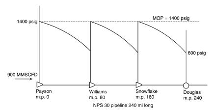
**Figure 2.** An illustration of compressor spacings in pipeline capacity increment (maximum operating pressure—MOP) [12].
