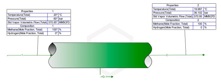
Figure 5. Existing pipeline single-pipe model diagram (\* denoting a feed stream).
