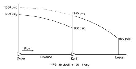
Figure 1. Pipeline expansion through inlet pressure increase [12].
