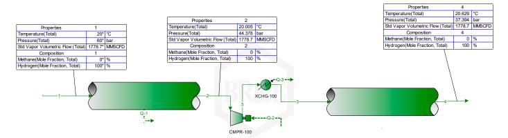
**Figure 8.** Process diagram for gas network expansion through compression (\* denoting a feed stream and -3- refers to the stream after heat exchanger XCHG-100).
