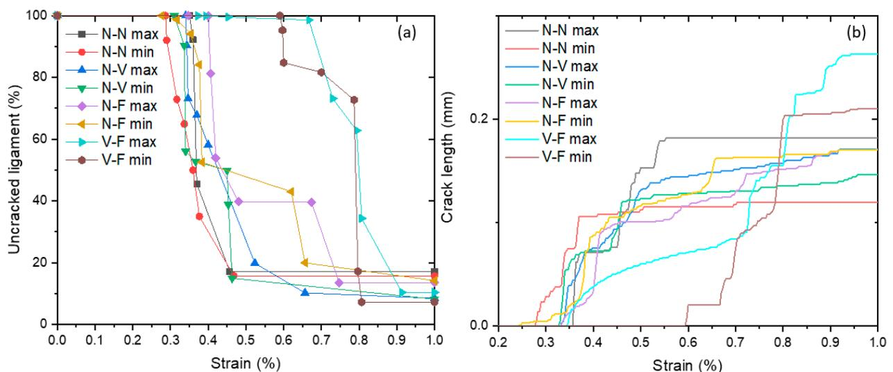
**Figure 13.** Evolution of uncracked ligament (a) and crack length (b) for different morphologies of graphite inclusions in tow-particle models and distances between them.
