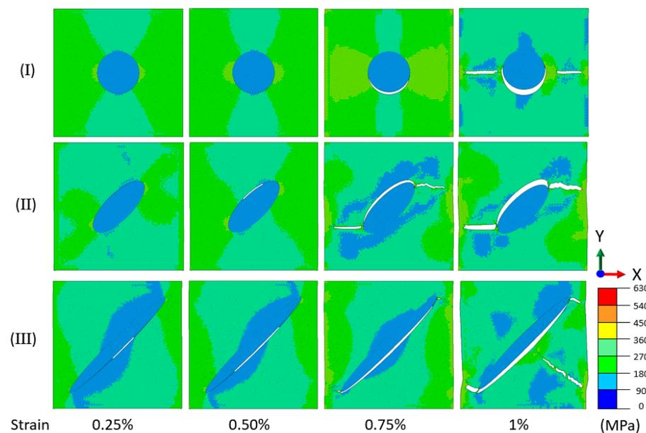
**Figure 7.** Evolution of von Mises stress distribution and crack growth under vertical tensile loading for different graphite morphology: (I) nodular; (II) vermicular; (III) flake.
