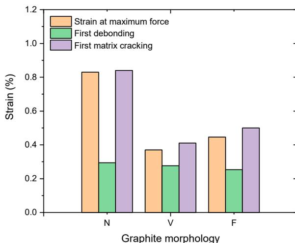
**Figure 9.** Main stages of crack propagation in terms of applied displacement for different graphite morphology (N—nodular, V—vermicular, F—flake).
