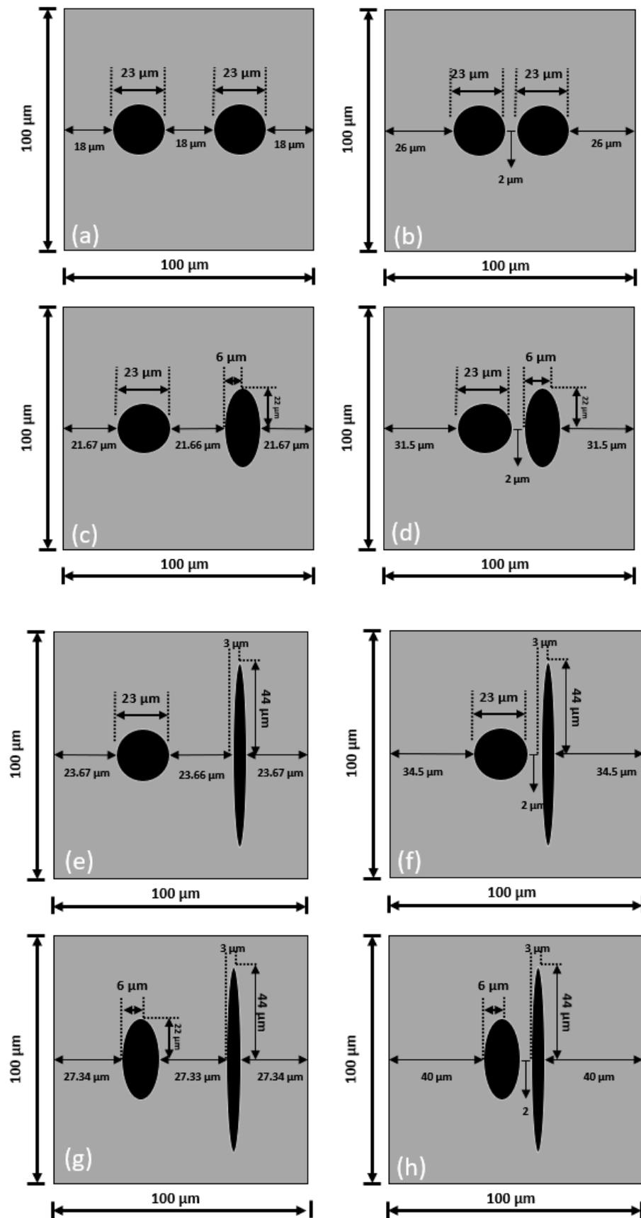
Figure 4. Geometrical parameters of unit cells for analysis of particle interaction: (a,c,e,g) maximum distance; (b,d,f,h) minimum distance.
