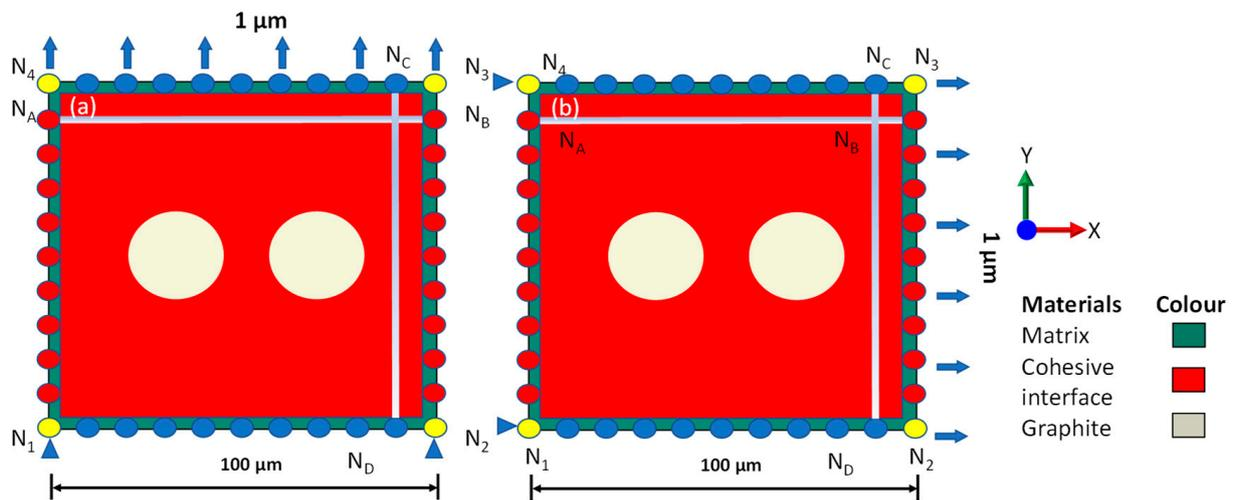
**Figure 5.** Schematics of PBCs with CZM under vertical (a) and horizontal (b) loading regimes.
