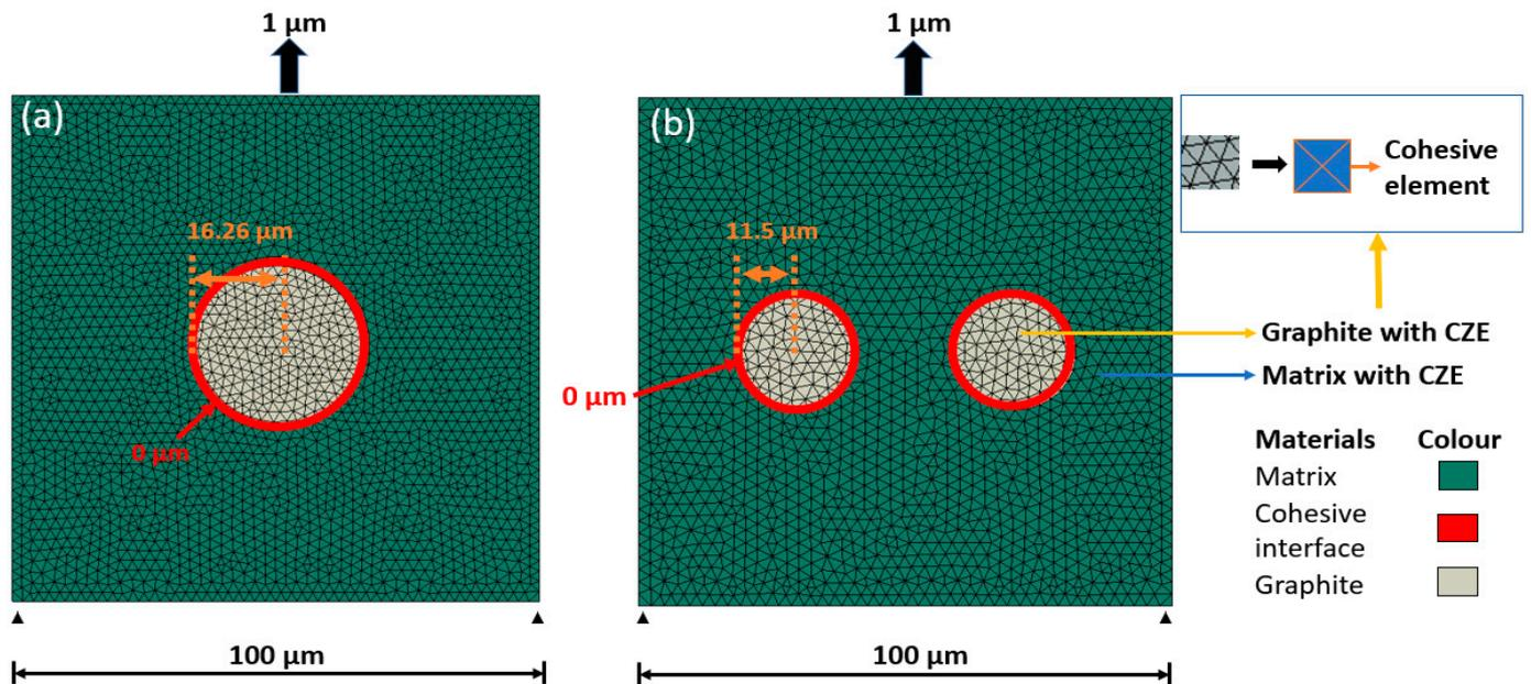
Figure 2. Geometry and mesh used in numerical simulations: (a) Single inclusion; (b) two inclusions.
