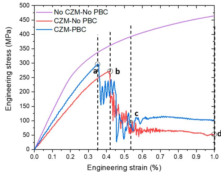
**Figure 11.** Effect of boundary conditions and CZM on macroscopic engineering stress–strain curve of CGI.
