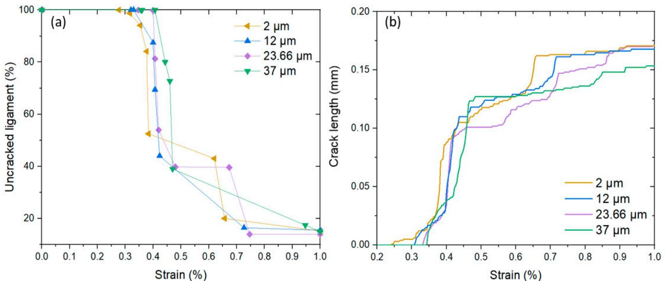
**Figure 15.** Effect of inter-particle spacing on evolution of uncracked ligament (a) and crack length (b) for N-F combination.
