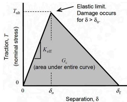
**Figure 6.** Traction–separation relationship (Reprinted with permission from Ref. [35]. 2016, D. Zhang).
