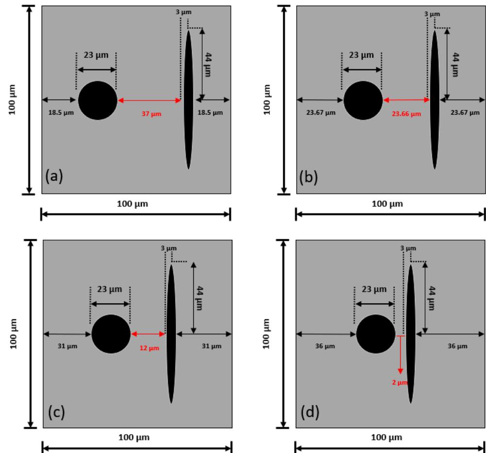
**Figure 14.** Geometrical parameters of unit cells for N-F models with different distances between particles: (a) 37  $\mu\text{m}$ ; (b) 23.66  $\mu\text{m}$ ; (c) 12  $\mu\text{m}$ ; (d) 2  $\mu\text{m}$ .
