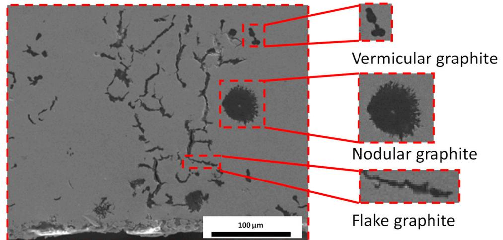
**Figure 1.** Microstructure of CGI.
