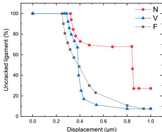
**Figure 8.** Effect of graphite morphology on evolution of uncracked-ligament length with external displacement (N—nodular, V—vermicular, F—flake).
