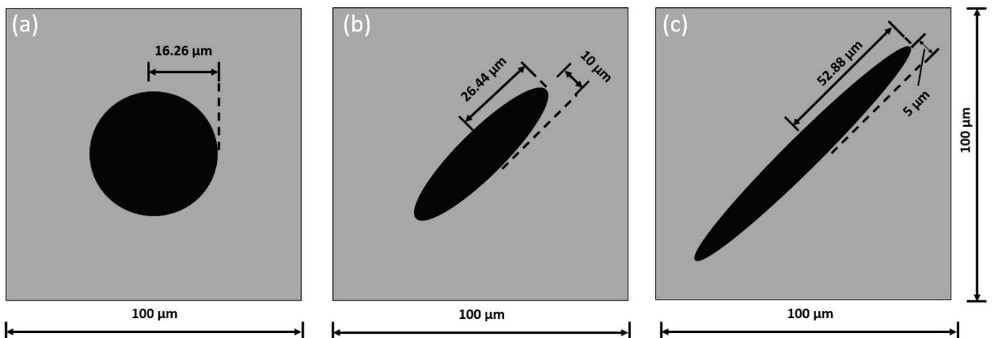
Figure 3. Geometry of nodular (a), vermicular (b), and flake (c) inclusions.
