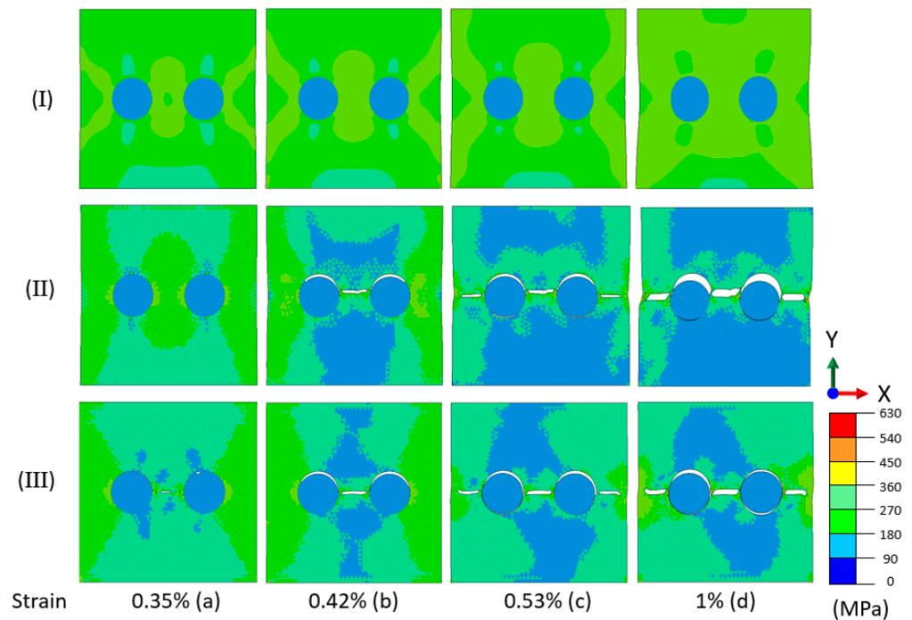
**Figure 10.** Crack propagation and von Mises stress distribution for vertical tensile loading in CGI for various cases of formulation: (I) without CZM; (II) with CZM; (III) CZM-PBCs.
