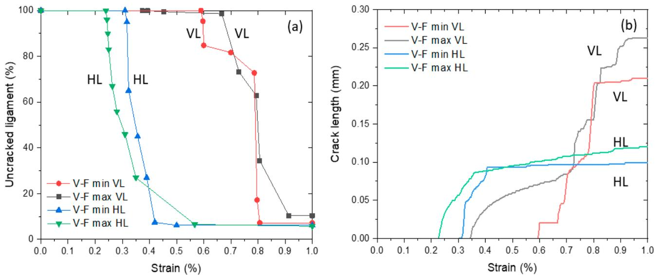
**Figure 17.** Evolution of uncracked ligament (a) and crack length (b) for different loading directions for two-particle V-F model with different spacings (VL—vertical loading; HL—horizontal loading).
