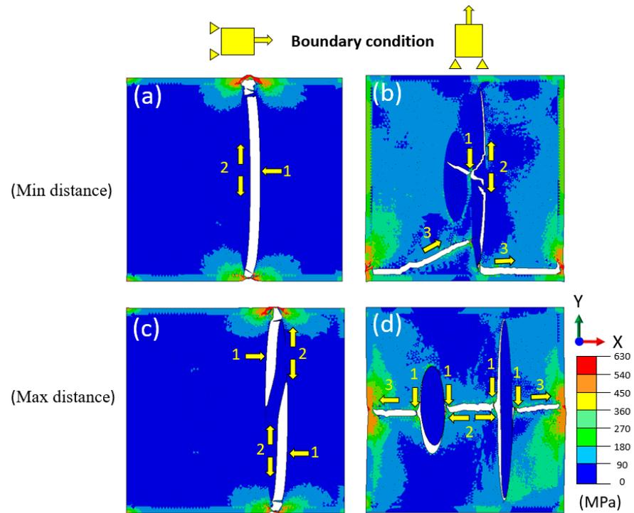
**Figure 16.** Crack propagation and von Mises stress distribution in CGI under horizontal (a,c) and vertical (b,d) loading regimes for two-particle V-F model with different spacings (1—crack initiation point; 2—beginning of crack propagation; 3—end of crack propagation).
