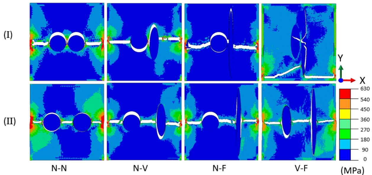
**Figure 12.** Crack propagation and von Mises stress distribution for vertical tensile loading in CGI for various graphite distances and particle morphologies: (I) minimum spacing; (II) maximum spacing (N—nodular, V—vermicular, F—flake).
