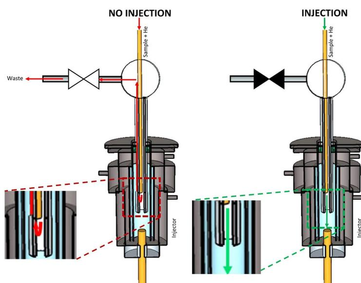
**Figure 2.** Scheme of multiplex injector design A. The green and red arrows indicate the flow of the carrier gas stream (transporting the sample) into and out of the GC's split/splitless injector when the sample was introduced ('Injection') or not ('No injection'). ►◄ represents a solenoid valve in the 'closed' state, while ▷◁ represents the valve in the 'open' state.
