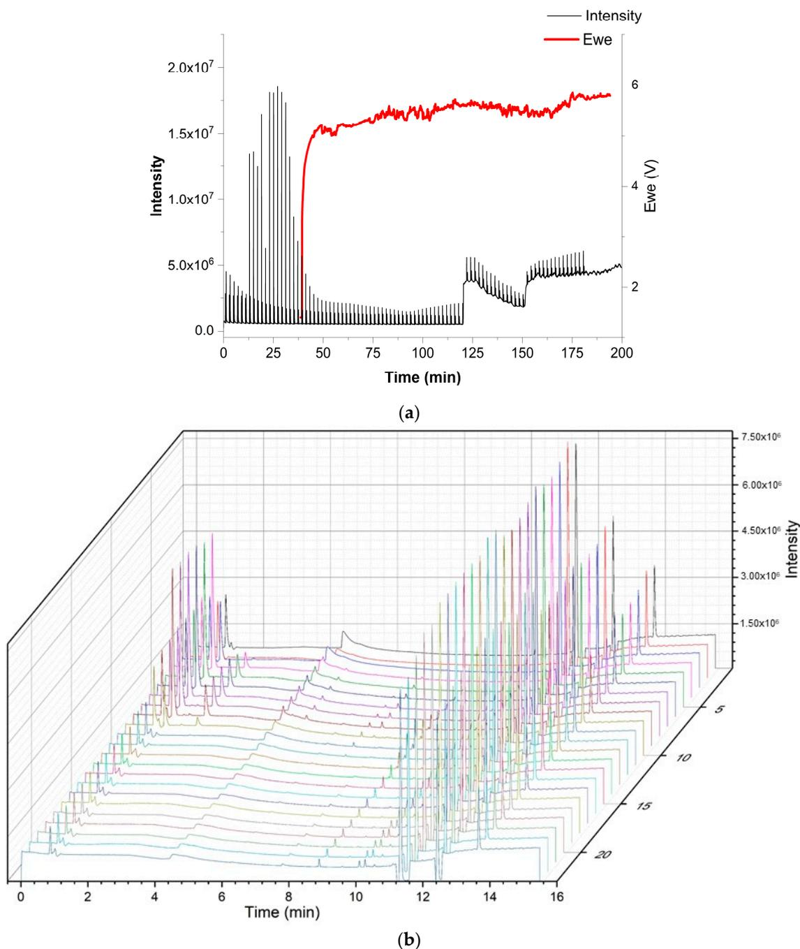
**Figure 11.** Real lithium-ion battery testing experiment of NMC 111 cell with the design C (a) (top) multiplexing and (b) (bottom) normal gradient conditions during overcharge. ( $E_{we}$ : potential of a working electrode in V).
