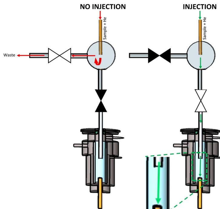
**Figure 3.** Scheme of multiplex injector design B. The green and red arrows indicate the flow of the carrier gas stream (transporting the sample) into and out of the GC's split/splitless injector when the sample was introduced ('Injection') or not ('No injection').  $\blacktriangleright\blacktriangleleft$  represents a solenoid valve in the 'closed' state, while  $\triangleright\triangleleft$  represents the valve in the 'open' state.
