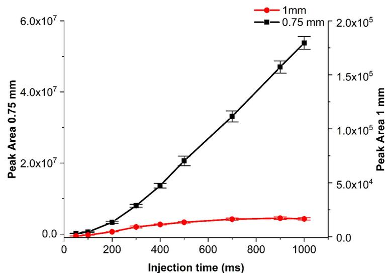
**Figure 7.** Comparison of the heptane peak area for two Tee connector bore sizes (1 and 0.75 mm) with increasing injection time for design B. The isothermal method is mentioned in Section 3.3 with a  $7\text{-mL min}^{-1}$  sample flow. Error bars indicate  $\pm 1$  s.
