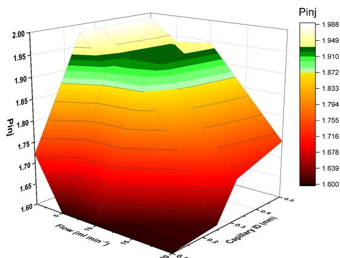
**Figure 5.** Interrelationship between sample flow rate, capillary ID and required injection pressure  $P_{\text{inj}}$  (in bar) for successful sample introduction.
