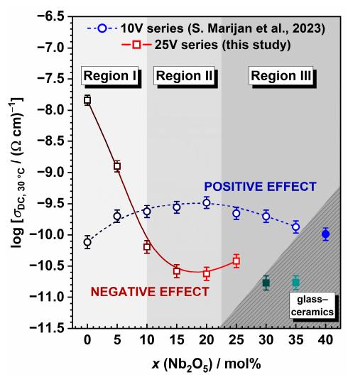
**Figure 8.** Comparison of compositional dependence of DC conductivity,  $\sigma_{DC}$ , at 303 K for two glass and glass-ceramics series,  $35Na_2O-10V_2O_5-(55 - x)P_2O_5 - xNb_2O_5$  [27] and  $35Na_2O-25V_2O_5-(40 - x)P_2O_5 - xNb_2O_5$ . The lines connecting data points are a guide for the eye.
