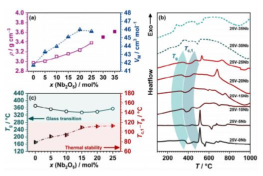
**Figure 1.** (a) Dependence of density,  $\rho$ , and molar volume,  $V_{\rm M}$ , on Nb<sub>2</sub>O<sub>5</sub> content; (b) DTA curves; and (c) dependence of glass transition temperature,  $T_{\rm g}$ , and the parameter ( $T_{\rm c} - T_{\rm g}$ ) on Nb<sub>2</sub>O<sub>5</sub> content. The lines connecting data points in (**a**,**c**) are a guide for the eye.
