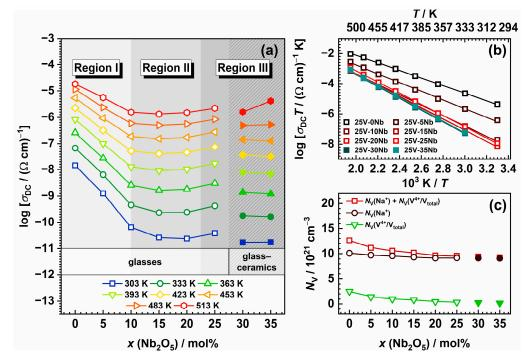
**Figure 6.** (a) Compositional and temperature dependence of DC conductivity,  $\sigma_{DC}$ ; (b) Arrhenius plot of DC conductivity; and (c) compositional dependence of number density,  $N_V$ , of Na<sup>+</sup> ions, V<sup>4+</sup> ions, and the total number density of charge carriers. Empty symbols represent glasses, whereas full symbols denote glass–ceramics. The lines connecting data points in (a,c) are a guide for the eye, while the lines in (b) are obtained through linear regression.
