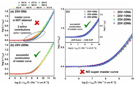
**Figure 7.** Summerfield scaling of conductivity spectra of (a) 25V-5Nb glass and (b) 25V-20Nb glass. (c) Construction of super master curve of the conductivity isotherms obtained by applying the Summerfield scaling procedure to all the investigated glasses; inset: individual master curves of glasses with  $10 \le x \le 25$  shifted along the x-axis to overlap with the reference master curve of 25V-10Nb glass.
