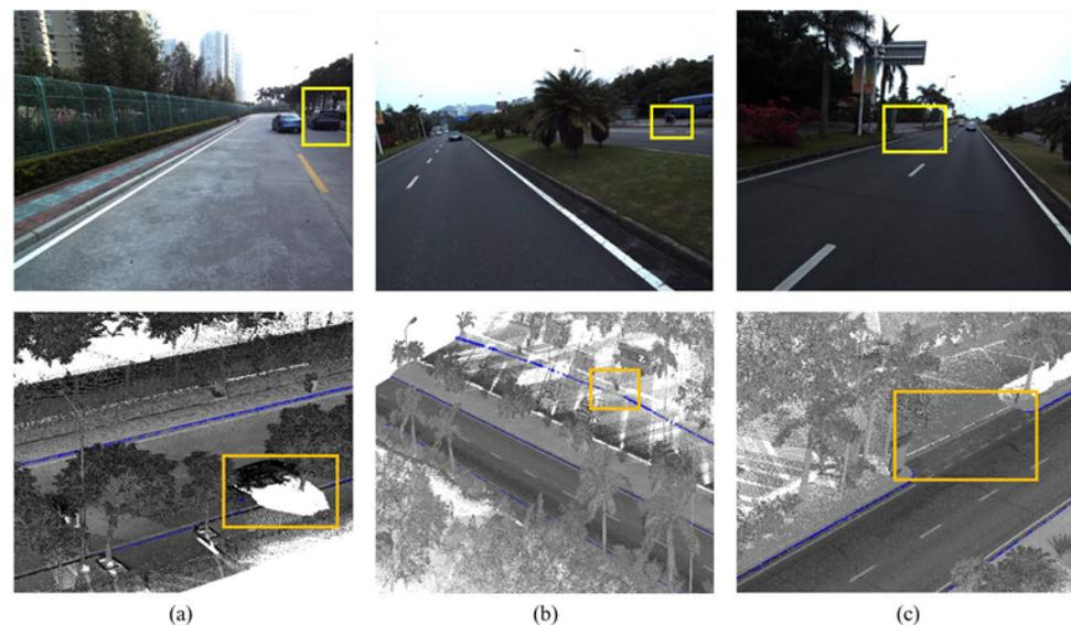
Figure 9. Curb detection using vision and LiDAR sensors: (a) Incomplete boundaries due to occlusions, (b) Worn road curbs, (c) A connection area between bikeways and roadways [42].
