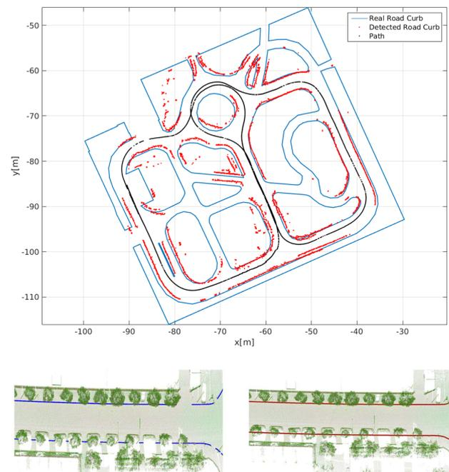
**Figure 17.** Curb mapping using a vision-based SLAM [1] and GPS [56].
