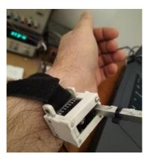
Figure 3. Application of the calorimeter on the wrist volar zone.
