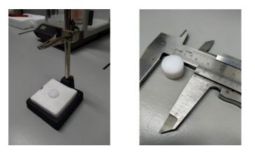
Figure 5. Small Teflon cylinder placed on a measurement base.
