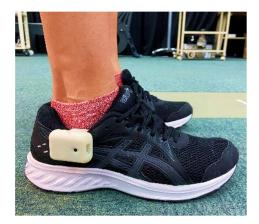
Figure 2. Auditory feedback device was attached on the lateral side of the shoe in the dominant leg.
