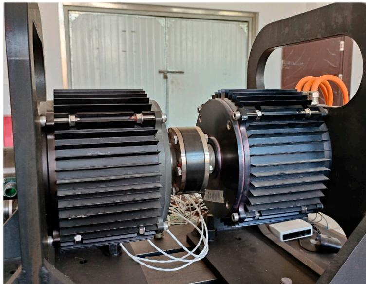
**Figure 4.** The prototype test platform of the 20p24s SPMSM.
