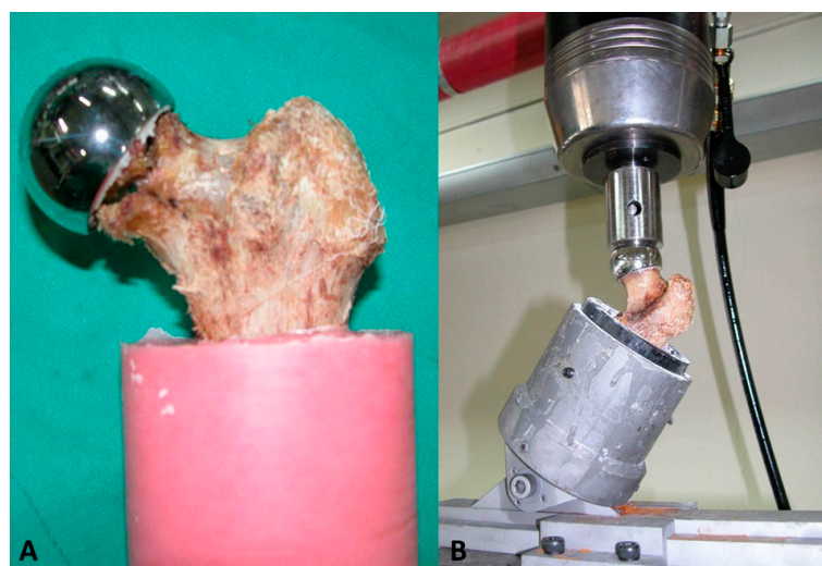
Figure 3. The preparation of the femoral specimens. (A) The femoral specimen was inserted in the resin block along the anatomical axis. (B) The femoral specimen with the femoral head implant was placed in a custom-made jig for the loading–unloading test.
