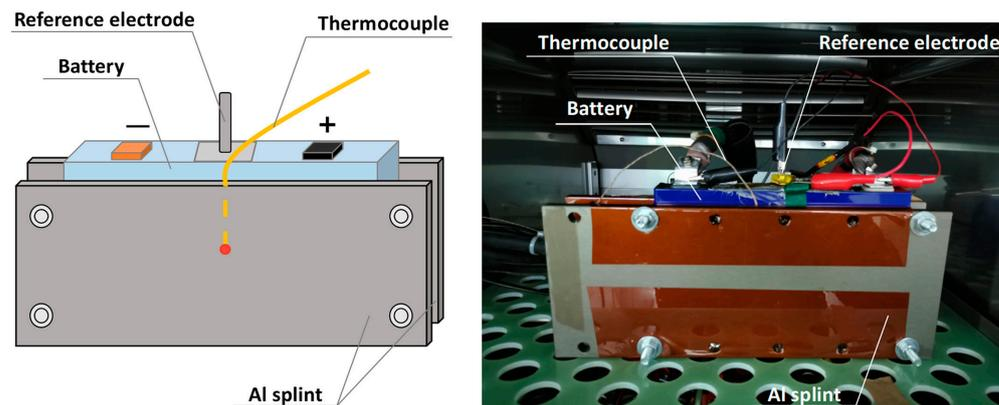
**Figure 2.** Sensing of internal electrode potential: high-capacity battery with built-in reference electrode and optimization of fast battery charging strategy based on reference electrode (reproduced with permission from Liu et al. International Journal of Energy Research; published by John Wiley and Sons, 2021) [16].
