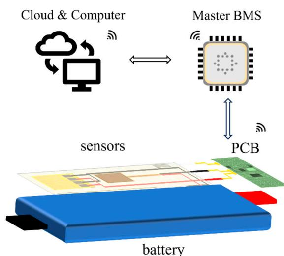
**Figure 1.** Schematic illustration of a smart battery equipped with multiple types of internal and external sensors.
