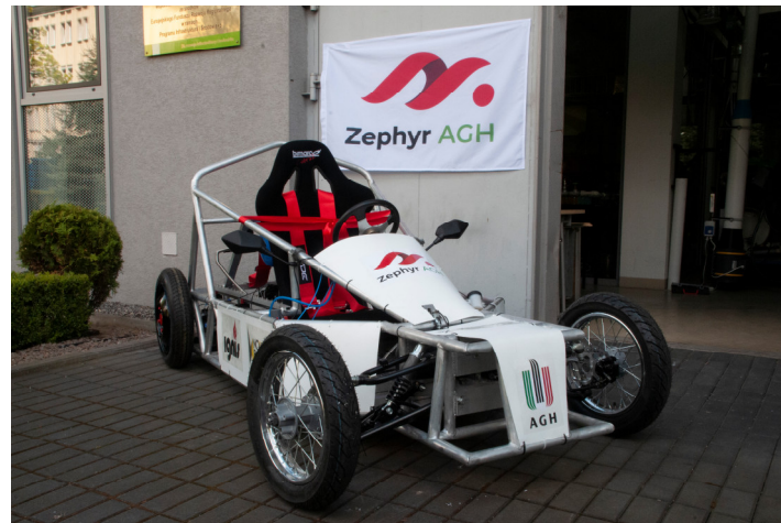
Figure 6. An example of a compressed air powered vehicle—the Zephyr AGH [82].
