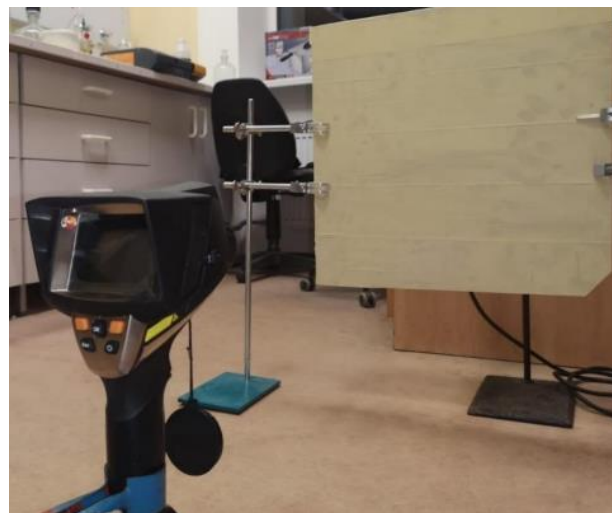
Figure 2. The setup of thermal transmittance experiment.
