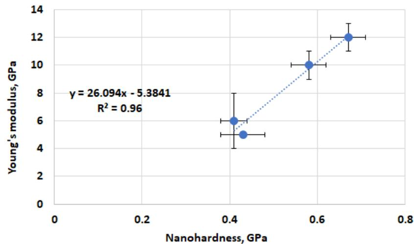
**Figure 10.** Young's modulus vs. nanohardness of ASR products (amorphous) of investigated mortars without additive and with 10%, 20%, and 30% calcined clay.
