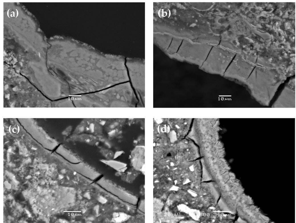
**Figure 5.** SEM-BSE micrograph of ASR products in air voids: (a) reference, (b) 10% calcined clay, (c) 20% calcined clay, and (d) 30% calcined clay.
