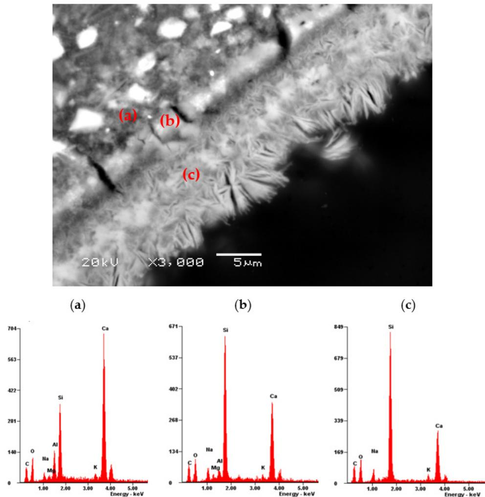
**Figure 6.** SEM-BSE micrograph with EDX analysis for the cement matrix and ASR products in an air voids in the mortar with 30% calcined clay: (a) cement matrix, (b) amorphous gel, and (c) crystalline gel.
