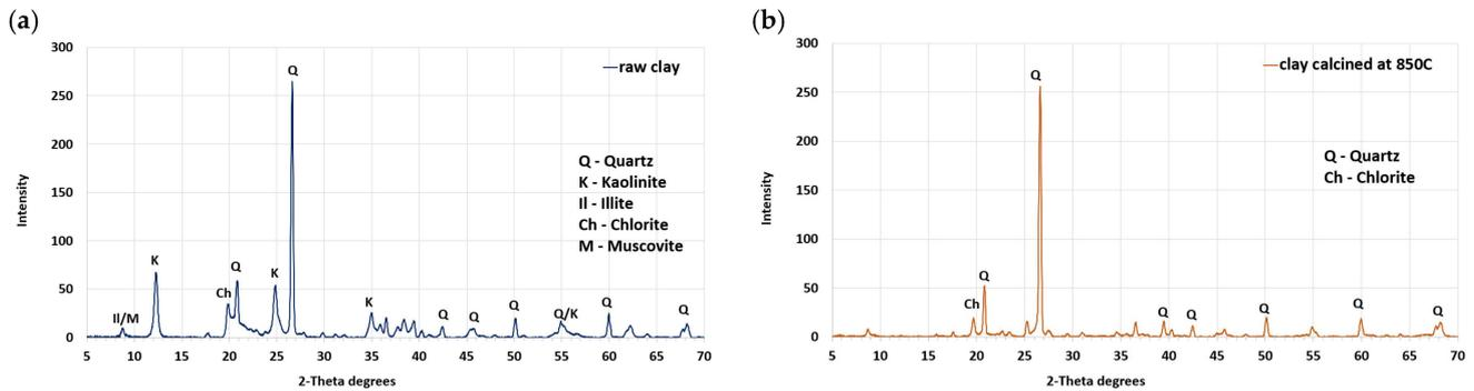
**Figure 1.** XRD patterns of (a) raw and (b) calcined clay.
