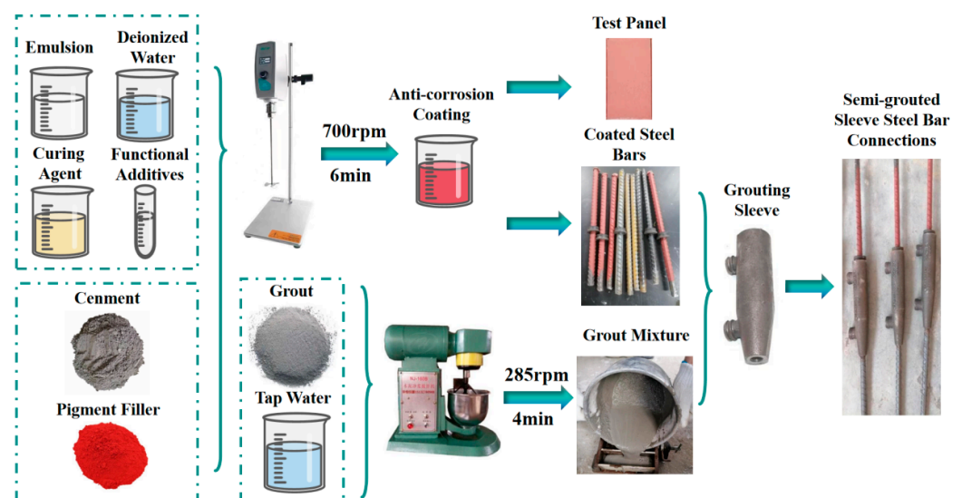
Figure 1. Samples and coated test panels preparation process.
