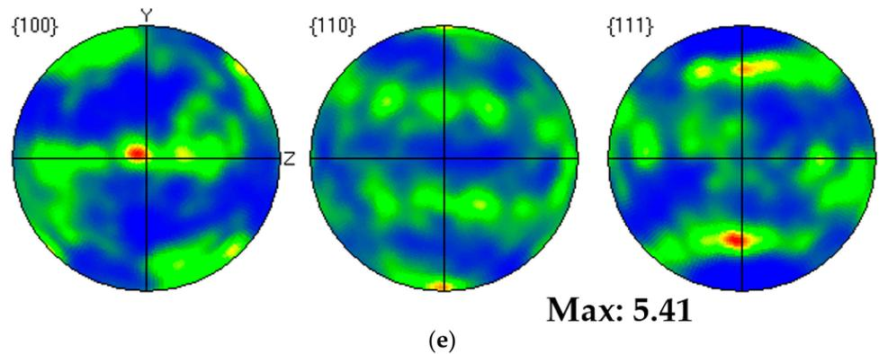
**Figure 20.** Texture analysis of Face 3: (a) IPF coloring map parallel to X; (b) IPF coloring map parallel to Y; (c) IPF coloring map parallel to Z; (d) IPF maps; (e) pole figures.
