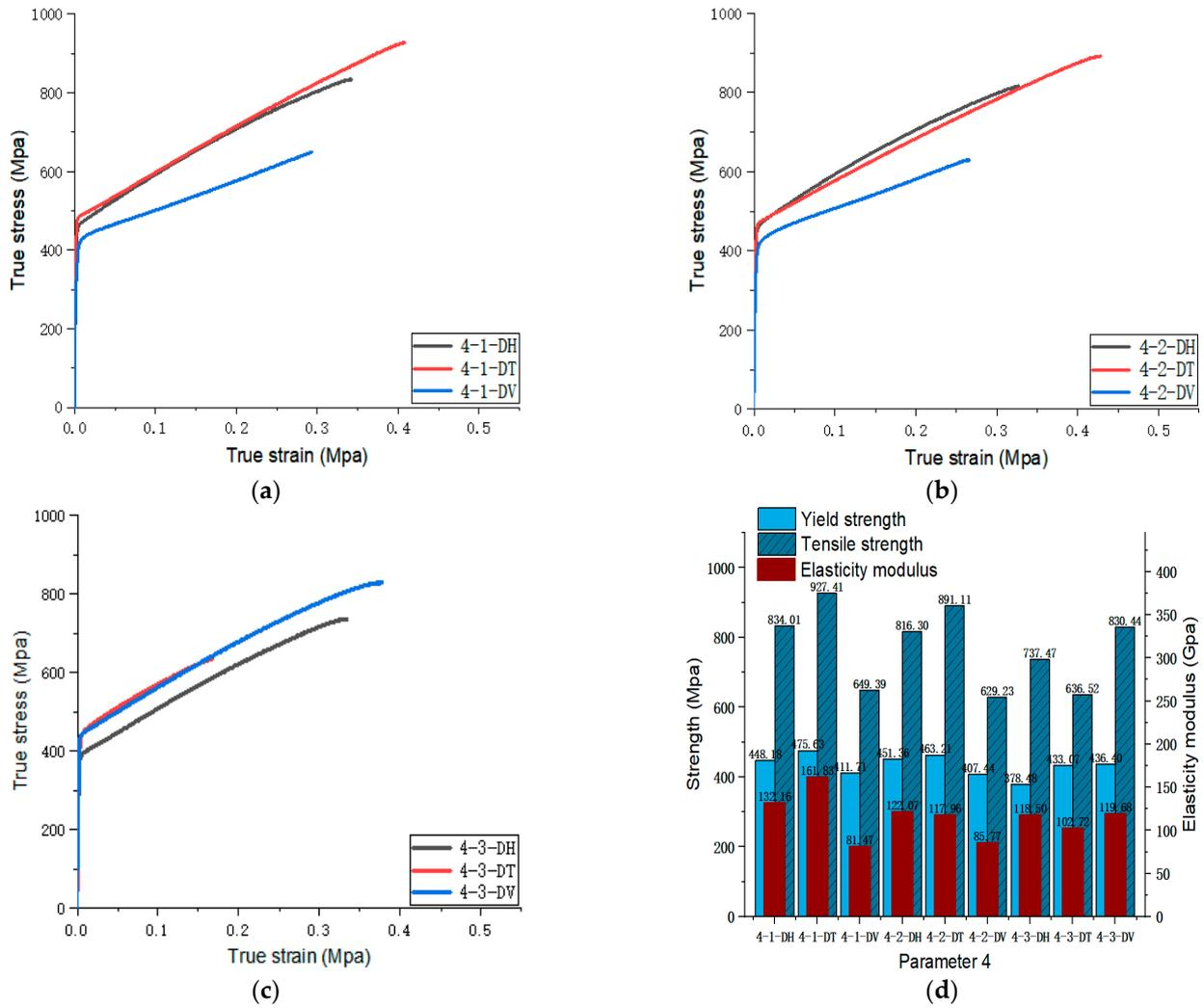
Figure 8. Parameter 4: (a) true stress-strain curves of three specimens on Face 1; (b) true stress-strain curves of three specimens on Face 2; (c) true stress-strain curves of three specimens on Face 3; (d) the yield strength, tensile strength, and elastic modulus of the specimen with parameter 4.
