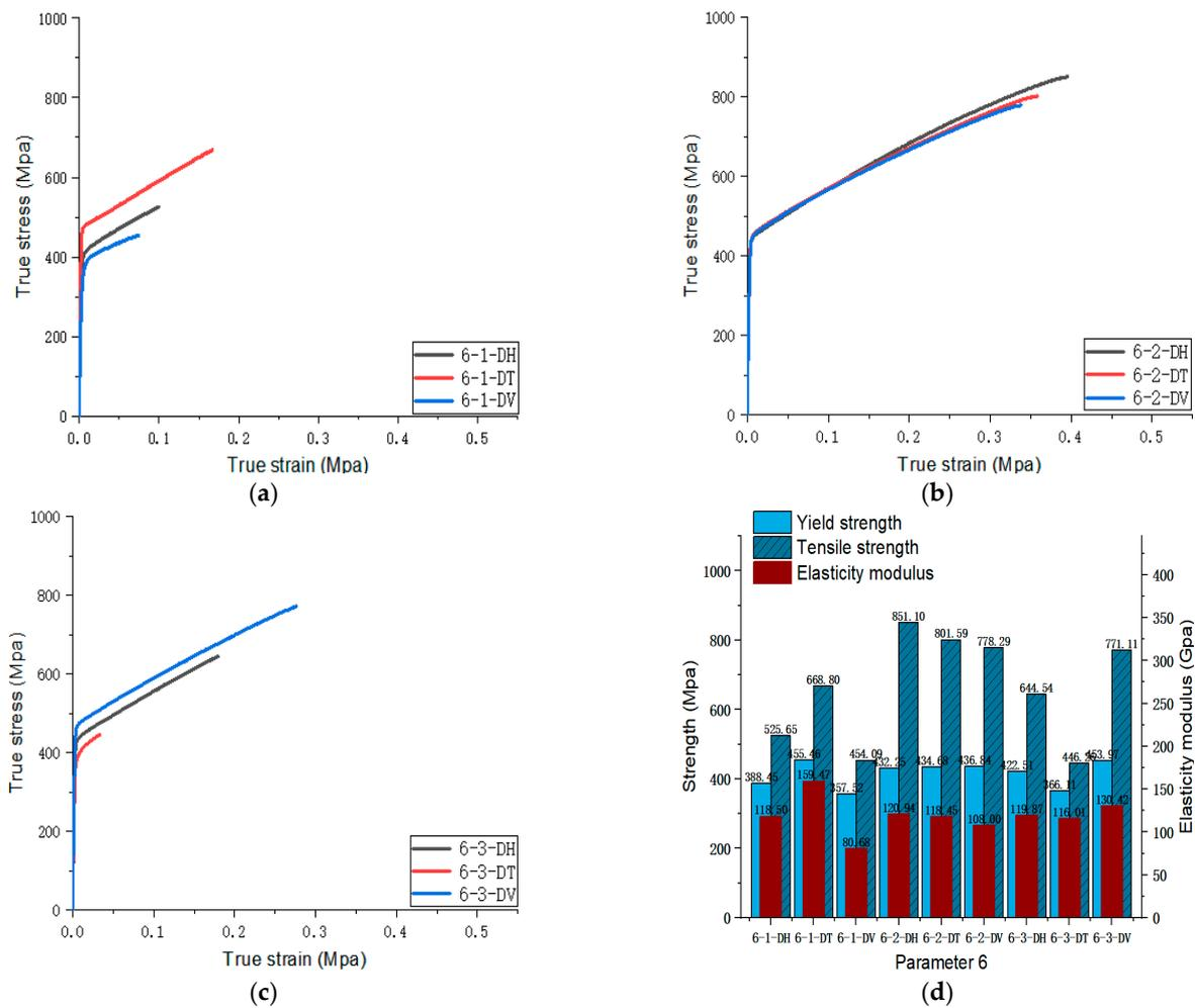
Figure 10. Parameter 6: (a) true stress-strain curves of three specimens on Face 1; (b) true stress-strain curves of three specimens on Face 2; (c) true stress-strain curves of three specimens on Face 3; (d) the yield strength, tensile strength, and elastic modulus of the specimen with parameter 6.
