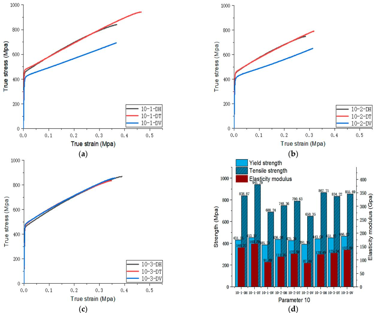
**Figure 14.** Parameter 10: (a) true stress-strain curves of three specimens on Face 1; (b) true stress-strain curves of three specimens on Face 2; (c) true stress-strain curves of three specimens on Face 3; (d) the yield strength, tensile strength, and elastic modulus of the specimen with parameter 10.
