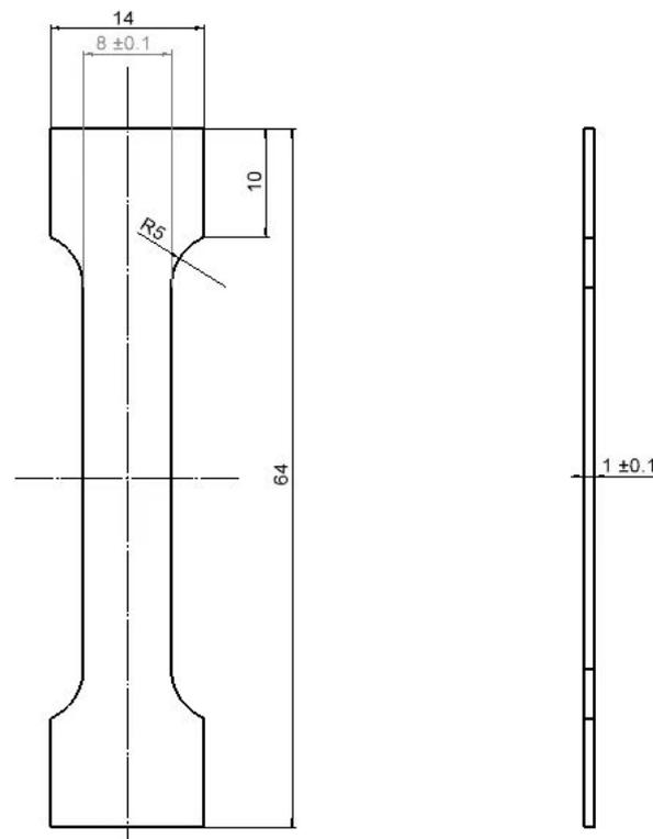
**Figure 3.** The specific size of uniaxial tensile specimen, Unit: mm.
