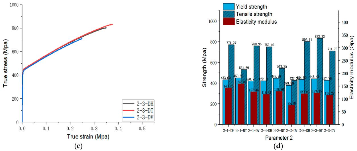
Figure 6. Parameter 2: (a) true stress-strain curves of three specimens on Face 1; (b) true stress-strain curves of three specimens on Face 2; (c) true stress-strain curves of three specimens on Face 3; (d) the yield strength, tensile strength, and elastic modulus of the specimen with parameter 2.
