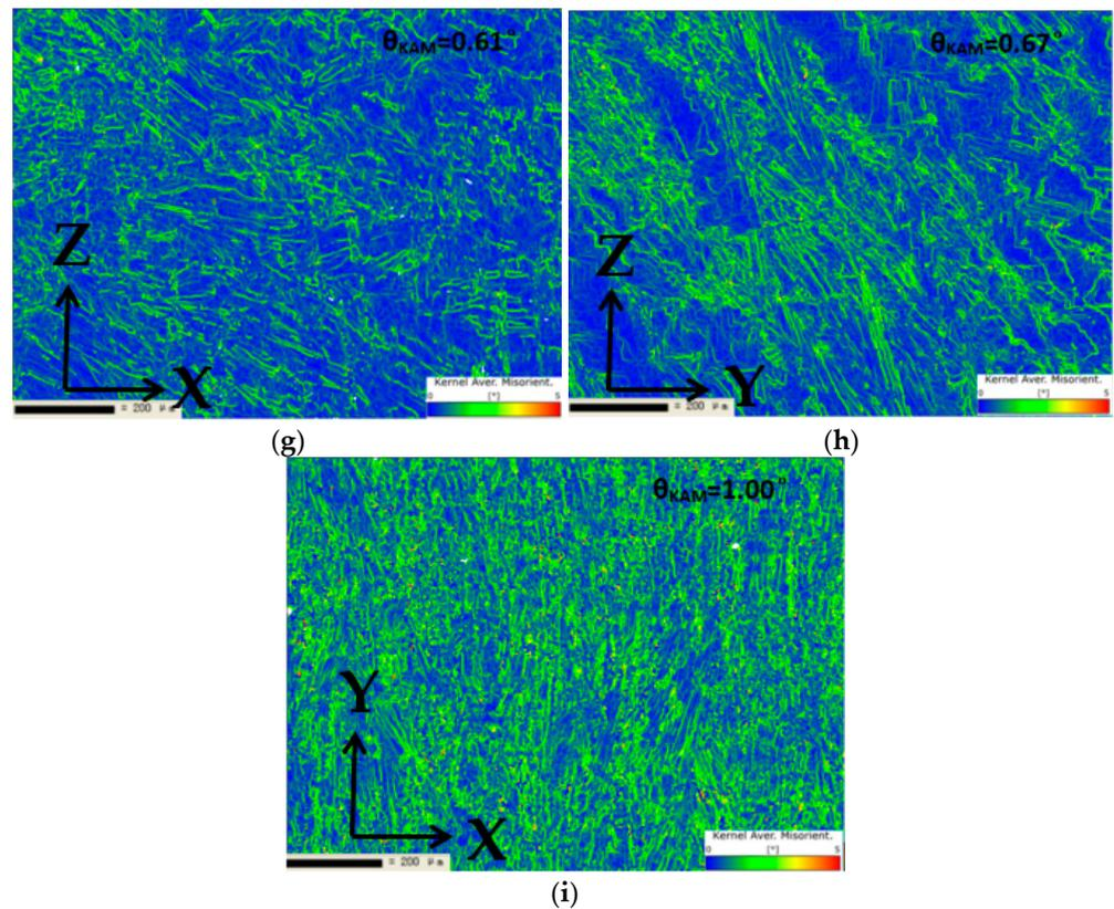
**Figure 17.** Microscopic analysis: (a) grain boundary figure of Face 1; (b) grain size distribution of Face 1; (c) grain boundary figure of Face 2; (d) grain size distribution of Face 2; (e) grain boundary figure of Face 3; (f) grain size distribution of Face 3; (g) kernel average misorientation figure of Face 1; (h) kernel average misorientation figure of Face 2; (i) kernel average misorientation figure of Face 3.
