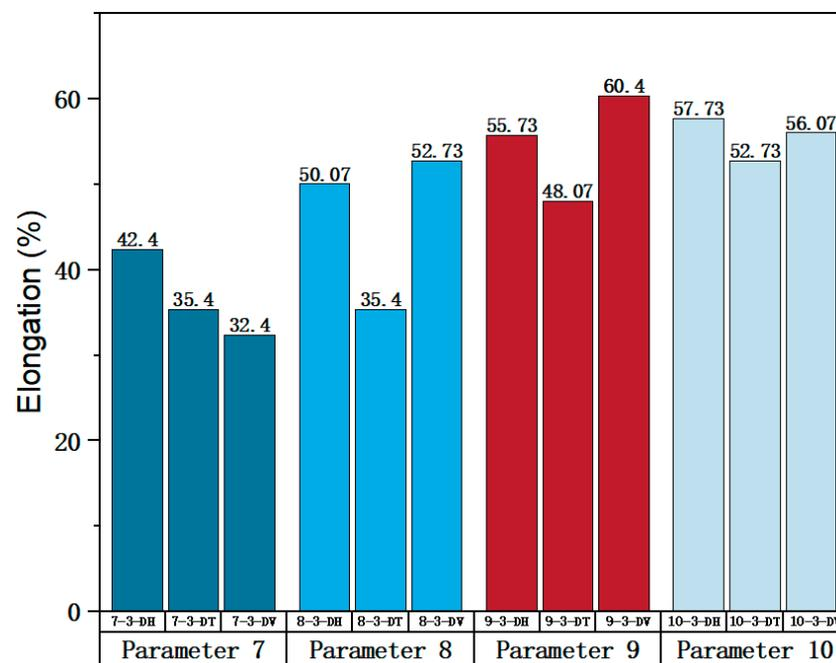
Figure 23. Elongation of the corresponding specimens.
