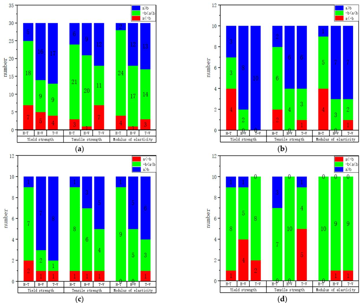
Figure 15. Statistical results of mechanical properties comparison of specimens with different directions on the same face: (a) complete specimens; (b) Face 1; (c) Face 2; (d) Face 3.
