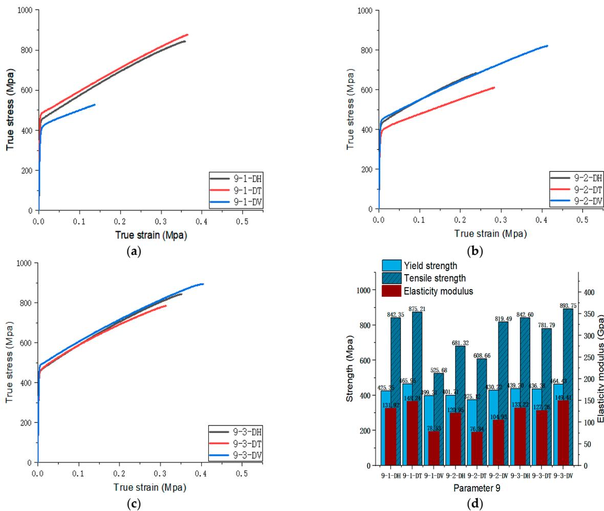
Figure 13. Parameter 9: (a) true stress-strain curves of three specimens on Face 1; (b) true stress-strain curves of three specimens on Face 2; (c) true stress-strain curves of three specimens on Face 3; (d) the yield strength, tensile strength, and elastic modulus of the specimen with parameter 9.
