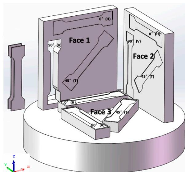
**Figure 2.** The printed sample and pick-up position.
