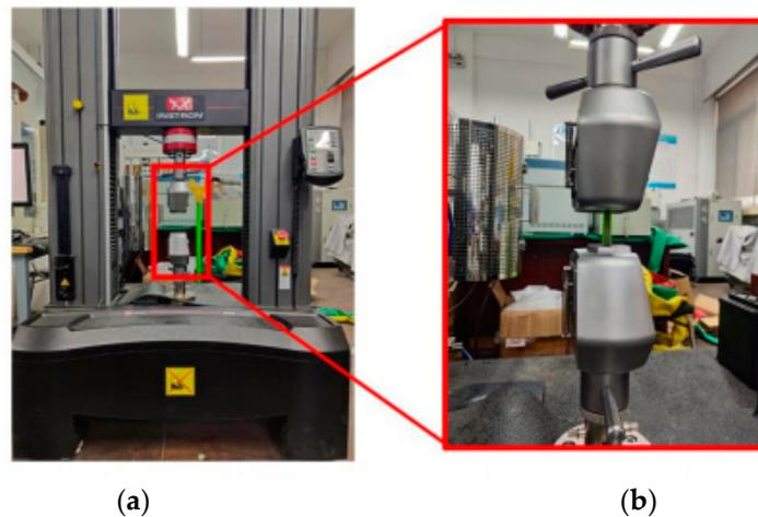
**Figure 4.** Intron universal testing machine. (a) Intron universal testing machine; (b) tester collet.
