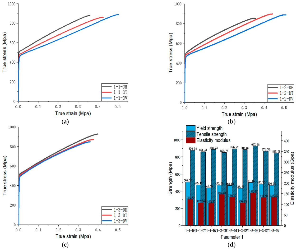
Figure 5. Parameter 1: (a) true stress-strain curves of three specimens on Face 1; (b) true stress-strain curves of three specimens on Face 2; (c) true stress-strain curves of three specimens on Face 3; (d) the yield strength, tensile strength, and elastic modulus of the specimen with parameter 1.
