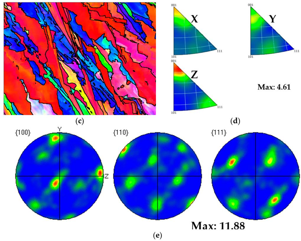
**Figure 19.** Texture analysis of Face 2: (a) IPF coloring map parallel to X; (b) IPF coloring map parallel to Y; (c) IPF coloring map parallel to Z; (d) IPF maps; (e) pole figures.
