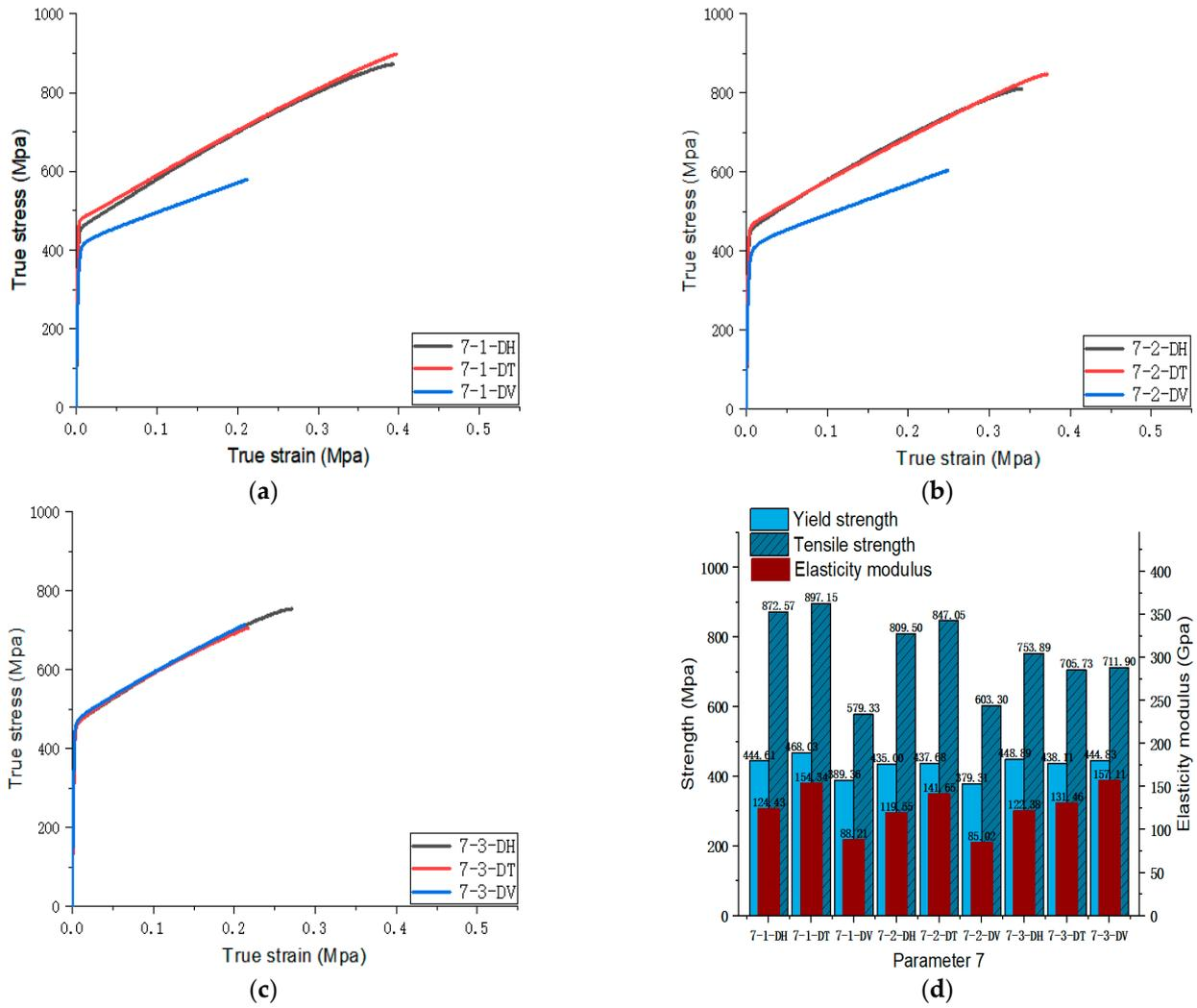
Figure 11. Parameter 7: (a) true stress-strain curves of three specimens on Face 1; (b) true stress-strain curves of three specimens on Face 2; (c) true stress-strain curves of three specimens on Face 3; (d) the yield strength, tensile strength, and elastic modulus of the specimen with parameter 7.
