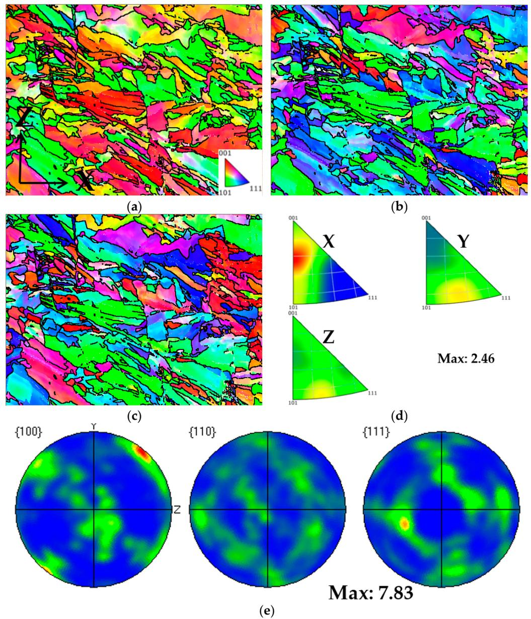
**Figure 18.** Texture analysis of Face 1: (a) IPF coloring map parallel to X; (b) IPF coloring map parallel to Y; (c) IPF coloring map parallel to Z; (d) IPF maps; (e) pole figures.
