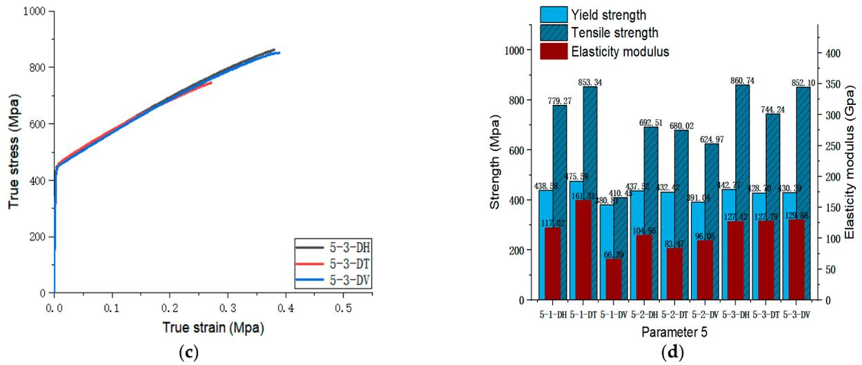
Figure 9. Parameter 5: (a) true stress-strain curves of three specimens on Face 1; (b) true stress-strain curves of three specimens on Face 2; (c) true stress-strain curves of three specimens on Face 3; (d) the yield strength, tensile strength, and elastic modulus of the specimen with parameter 5.
