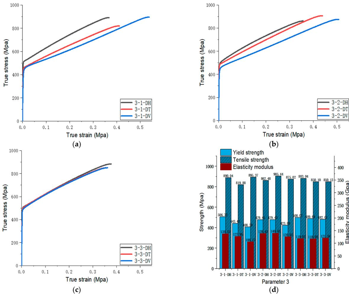
Figure 7. Parameter 3: (a) true stress-strain curves of three specimens on Face 1; (b) true stress-strain curves of three specimens on Face 2; (c) true stress-strain curves of three specimens on Face 3; (d) the yield strength, tensile strength, and elastic modulus of the specimen with parameter 3.
