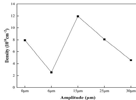
Figure 17. Curves of total dislocation density at different amplitude.
