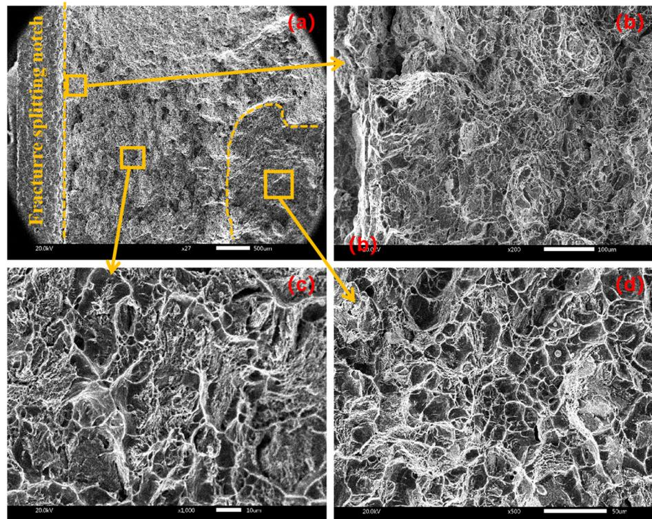
**Figure 10.** Fracture morphology at amplitude of 0  $\mu\text{m}$  with (a) macroscopic fracture, (b) crack initiation area, (c) extension area, (d) termination area.
