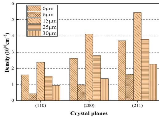
Figure 16. Dislocation density of different crystal planes at different amplitude.
