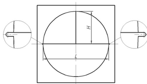
Figure 5. Definition of deformation.
