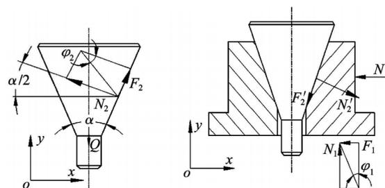
Figure 4. Schematic diagrams of force analysis of cracking unit.
