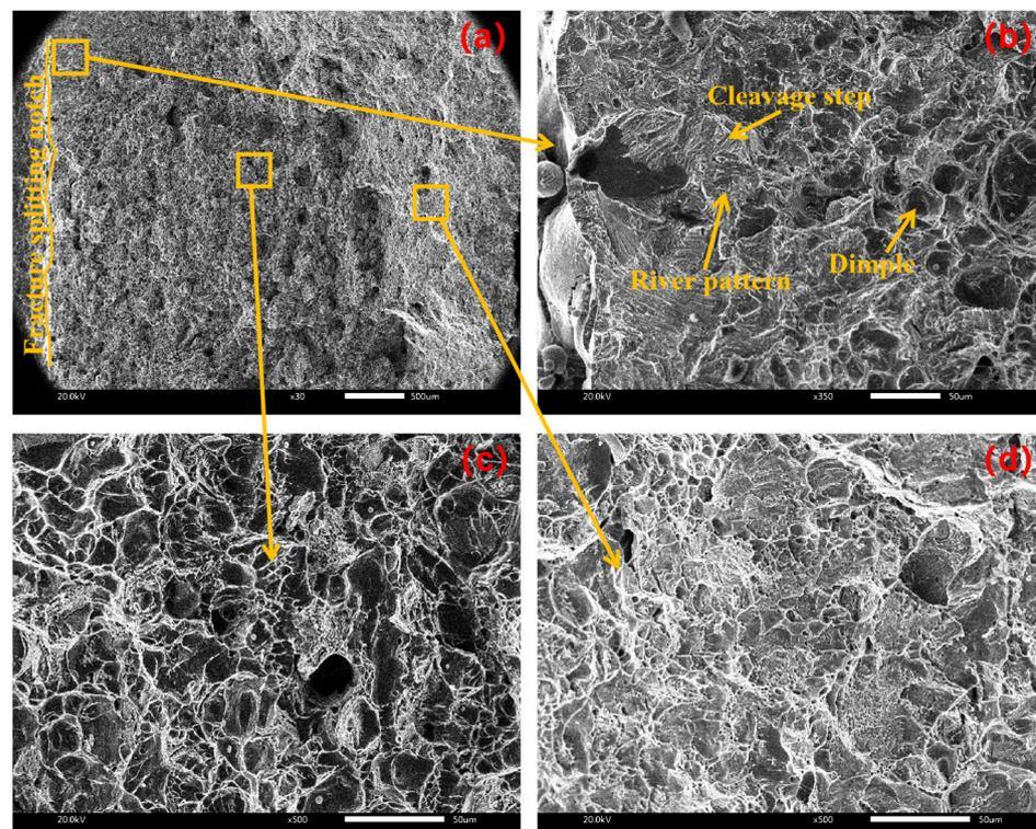
**Figure 11.** Fracture morphology at amplitude of 6  $\mu\text{m}$  with (a) macroscopic fracture, (b) crack initiation area, (c) extension area, (d) termination area.
