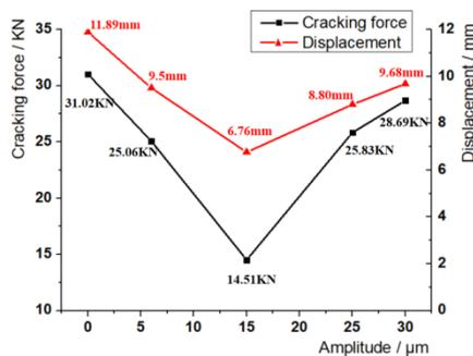
Figure 7. Amplitude–cracking force and amplitude–displacement curve.
