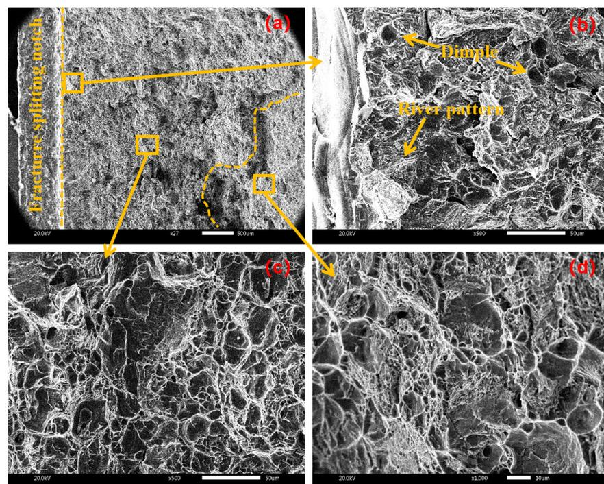
**Figure 14.** Fracture morphology at amplitude of 30  $\mu\text{m}$  with (a) macroscopic fracture, (b) crack initiation area, (c) extension area, (d) termination area.
