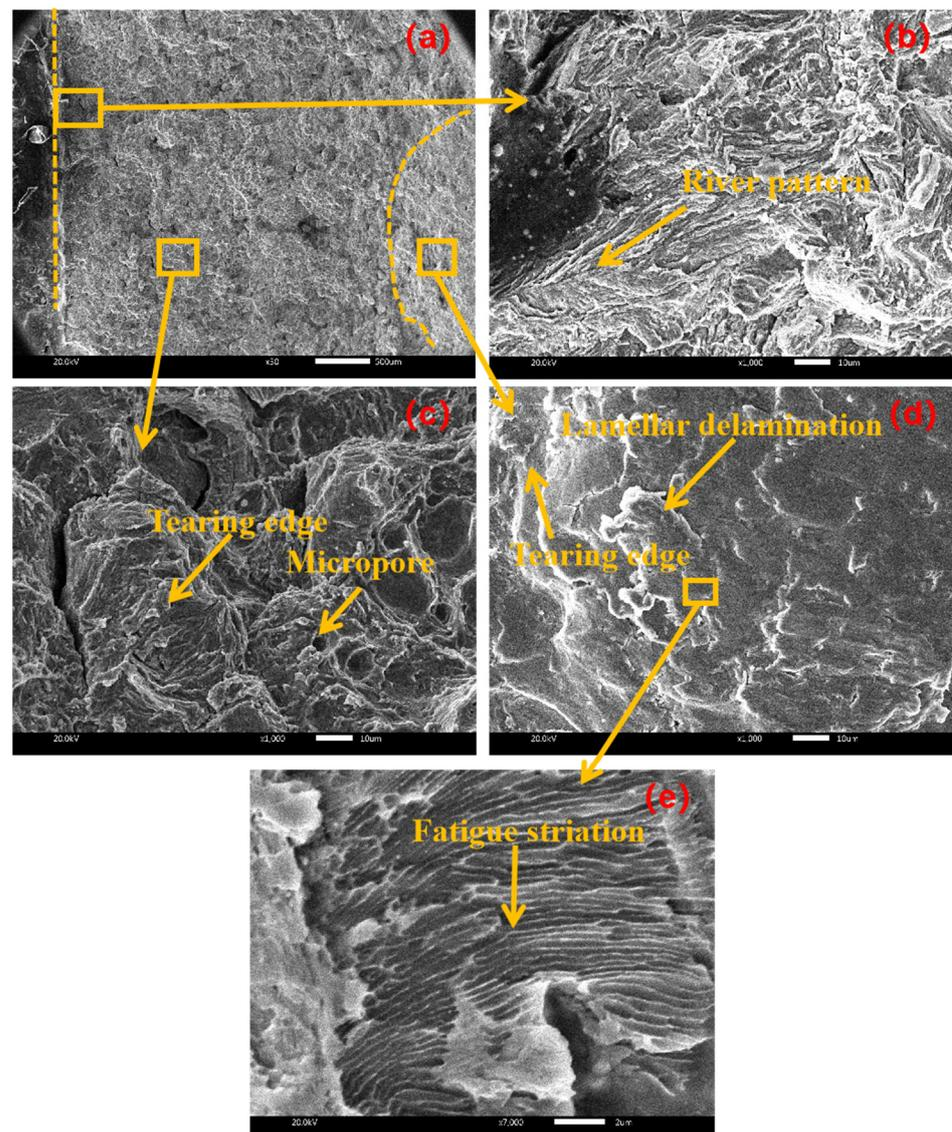
**Figure 12.** Fracture morphology at amplitude of 15  $\mu\text{m}$  with (a) macroscopic fracture, (b) crack initiation area, (c) extension area, (d) termination area (e) local magnification.
