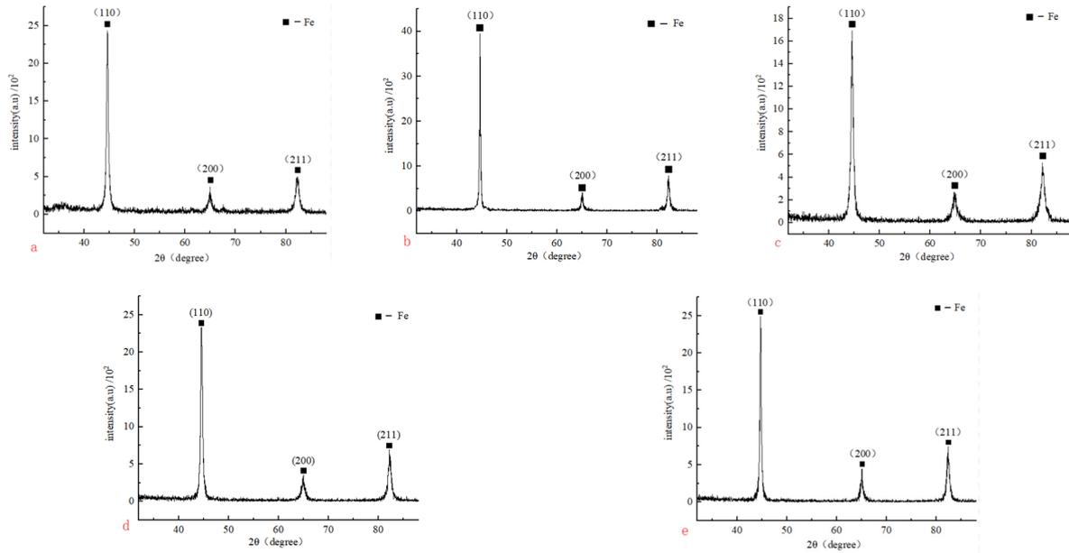
Figure 15. XRD pattern of sample fracture at different amplitude with (a) 0 μm, (b) 6 μm, (c) 15 μm, (d) 25 μm, (e) 30 μm.
