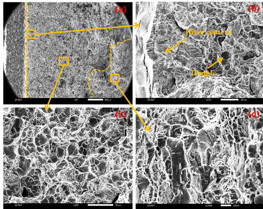
**Figure 13.** Fracture morphology at amplitude of 25  $\mu\text{m}$  with (a) macroscopic fracture, (b) crack initiation area, (c) extension area, (d) termination area.
