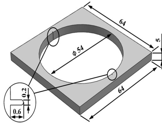
Figure 2. Cracking sample (unit: mm).
