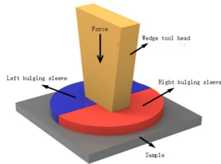
Figure 3. Schematic diagram of ultrasonic vibration-assisted cracking.
