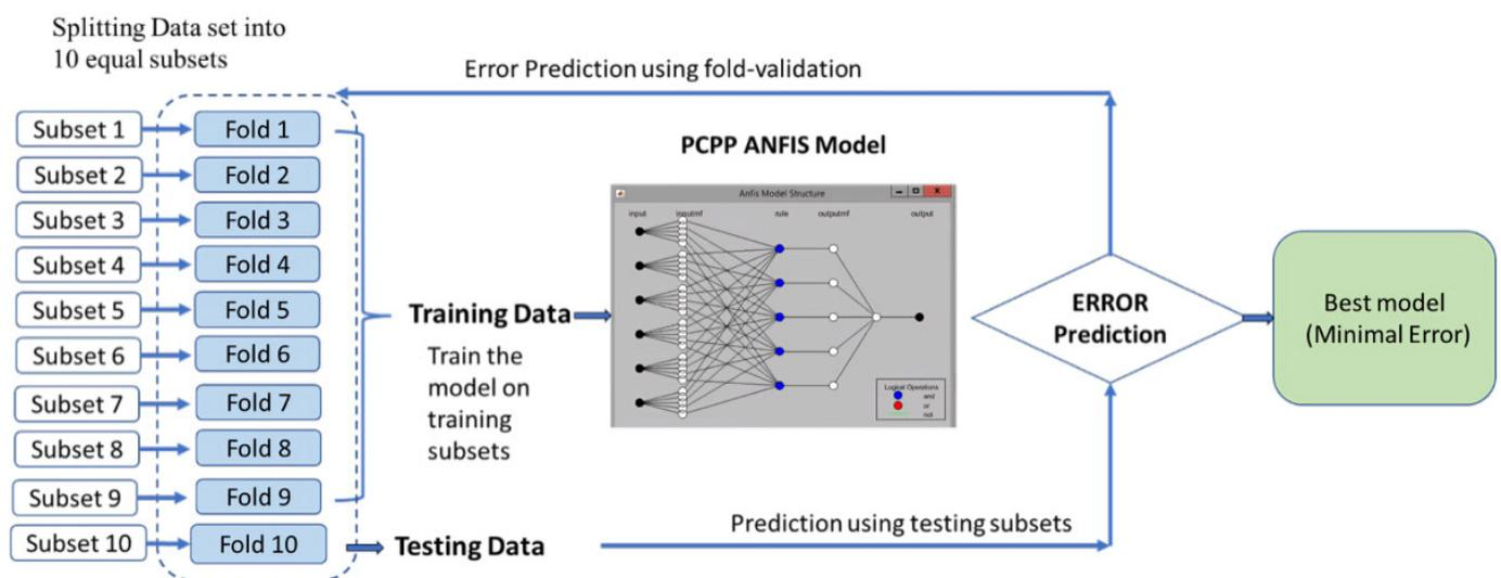
Figure 5. ANFIS–PCPP k-fold cross-validation diagram.
