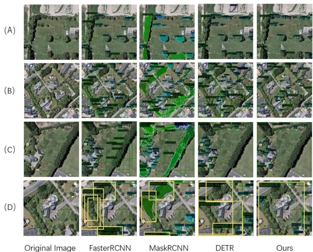
Figure 7. Comparison of detection performance for different networks. In rows (A–C), you can see a comparison of the detection results for different networks. The leftmost column shows the original image, while the following columns display the detection results of various networks. Row (D) is an enlarged view of the top left part of row (B), with highlighted bounding boxes to better visualize the results. Our method reduces the issue of duplicate detections.
