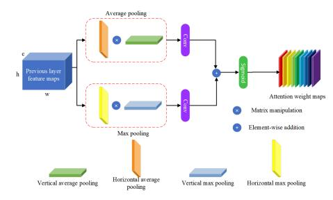
Figure 5. Parallel attention mechanism contains four types of pooling strategies.
