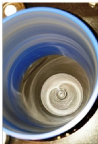
Figure 10. View of the B2 fluid spread evenly on the beaker walls.
