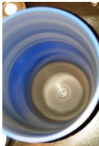
Figure 9. View of the potential vortex in fluid B2.
