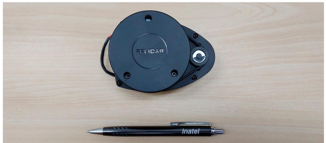
**Figure 3.** Slamtec LiDAR RPLiDAR A1 [53].
