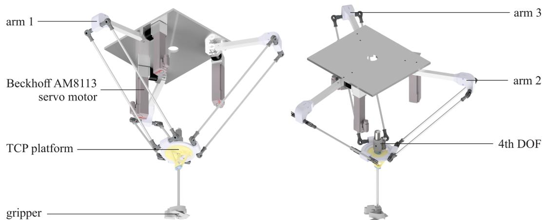
**Figure 1.** The delta robot consists of three parallel arms driven by servo motors, and an additional rotational axis for gripper orientation control.
