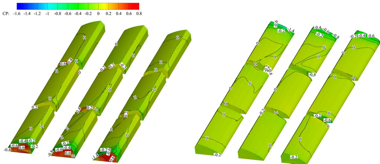
Figure 12. Cloud chart of wind pressure coefficient distribution on the surface of the solar greenhouse group.
