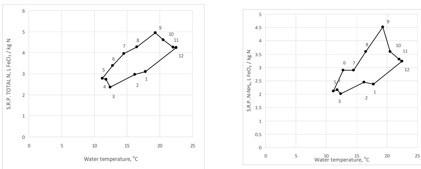
**Figure 8.** Correlations between water temperature and specific removal power for: **Left:** total nitrogen; **Right:** ammonia nitrogen.
