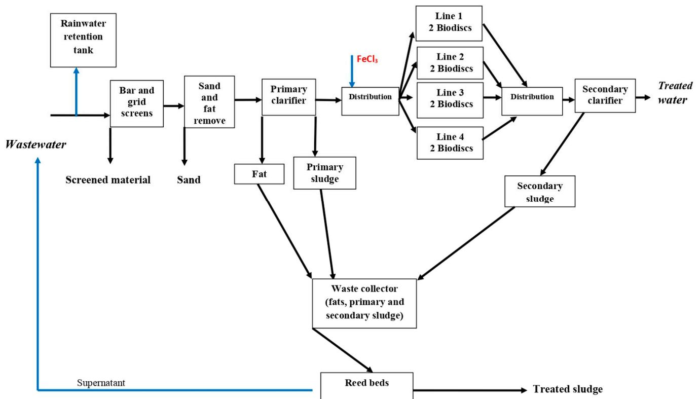
**Figure 1.** Flowchart of the Agnita WWTP.
