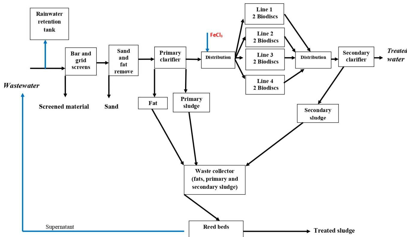
**Figure 1.** Flowchart of the Agnita WWTP.
