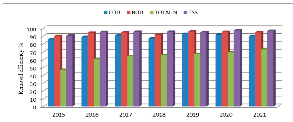
**Figure 3.** Removal efficiency for the main pollutants during the period 2015–2021.
