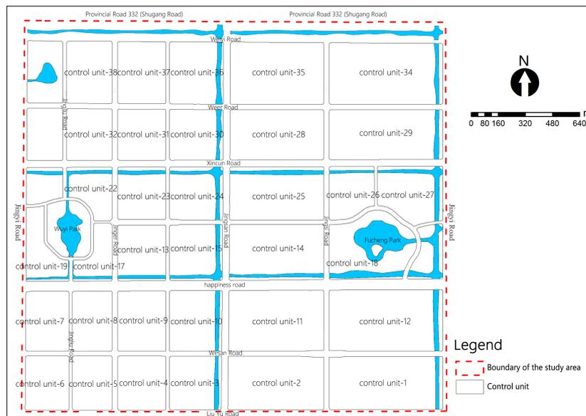
**Figure 3.** Low-impact development control unit division in the starting area of Yancheng Dafeng High-tech Zone.
